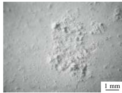
Fig.7 Morphology of the surface precipitates I: aggregated state
