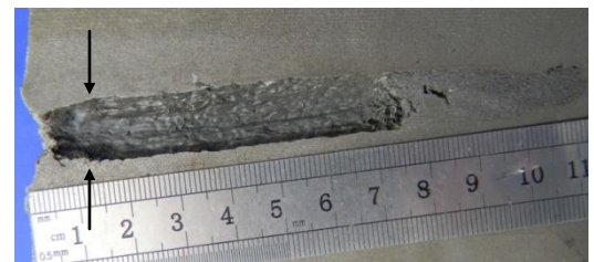
图 4 7#弹(复合材料)孔的线切割剖面照片 Fig.4 Picture of cross-section of 7# (composite, v=1634.8 m/s)
