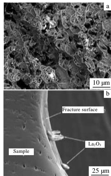
Fig.5 SEM images of high temperature fracture surfaces: (a) TMC3, 400 °C and (b) coarse La<sub>2</sub>O<sub>3</sub> reinforcement in TMC3, 500 °C
