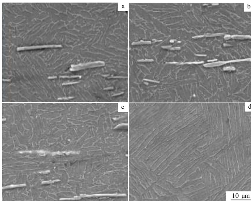
Fig.1 SEM images of the forged (TiB+La $_2$ O $_3$ )/Ti6Al4V matrix composite with addition of La and B element: (a) TMC1, (b) TMC2, (c) TMC3, and (d) matrix alloy
