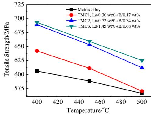
Fig.4 High temperature tensile strengths of (TiB+La<sub>2</sub>O<sub>3</sub>)/Ti6Al4V composites
