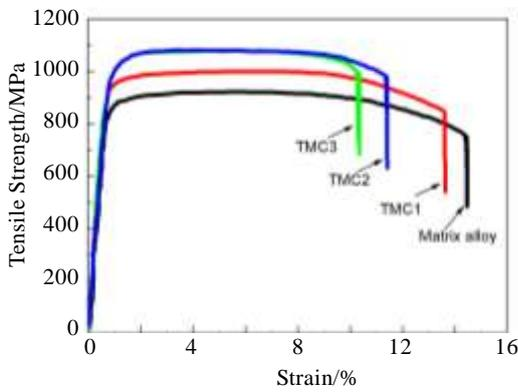
Fig.3 Tensile stress-strain curves of the specimens
