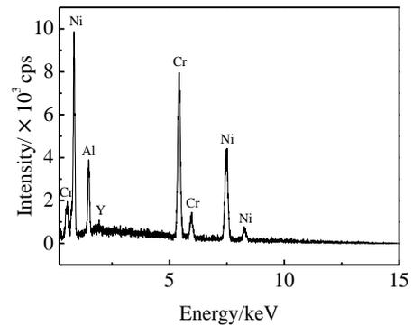
Fig.3 EDS spectrum of NiCrAlY coating
