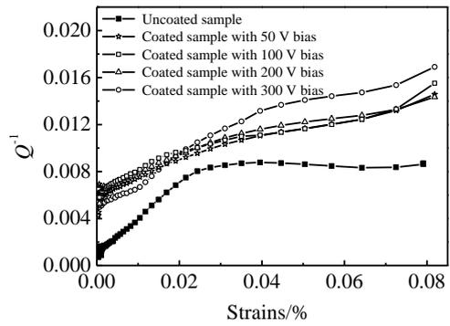
Fig.6 Variation of the samples damping capacity ( $Q^{-1}$ ) with the strains tested by DMA
