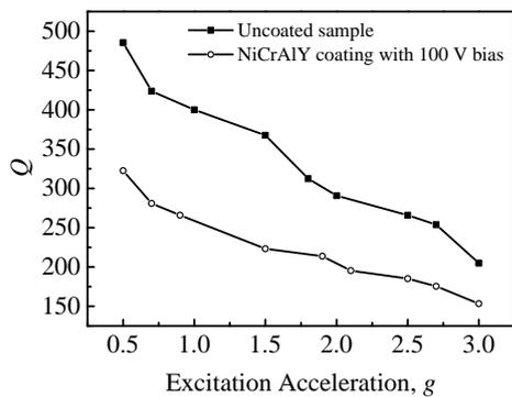
Fig.7 Variation of samples quality factor ( $Q$ ) with excitation force (g) tested by sine sweeps
