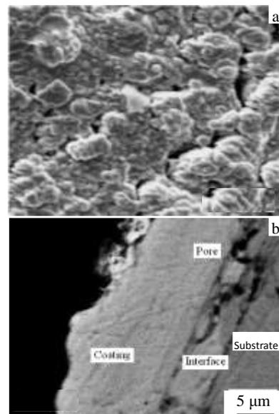
Fig.4 SEM morphologies of NiCrAlY coating surface (a) and cross-sectional (b)
