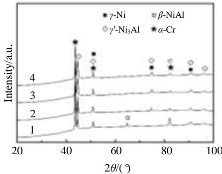
Fig.5 XRD patterns of NiCrAlY coating (1-sample with 50 V bias, 2-sample with 100 V bias, 3-sample with 200 V bias, 4-sample with 300 V bias)
