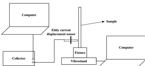
Fig.2 Schematic diagram of sine sweeps testing
