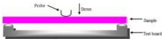
Fig.1 Schematic diagram of dynamic mechanical analyzer
