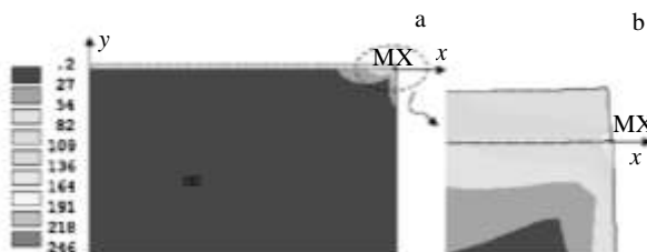
Fig.3 Typical contour of von Mises stress (MPa): (a) the whole region of the sample and (b) the local region near the edge of the coating and substrate interface
