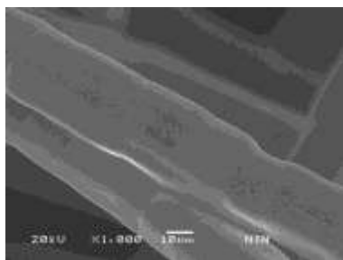
Fig.7 Sintered neck of two metal fibers with the fiber angle of 30 °
