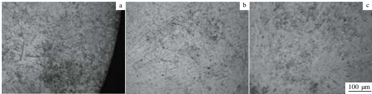
Fig.2 Metallographical structures of as-cast \text{Ti}_{40}\text{Ni}_{40}\text{Cu}_{20} ternary alloy: (a) edge region, (b) transition region, and (c) center region
