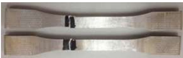
图 9 双杆进料的镁合金板材垂直于挤压方向试样断口位置 Fig.9 Fracture positions of the samples in TD of the magnesium sheets processed by the double rod mode
