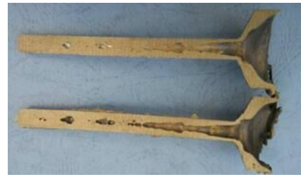
图 10 0.03 MPa 压差作用下单股液流吸铸成形排气阀 Fig.10 Exhaust valve formed by single strand liquid flow under 0.03 MPa differential pressure
