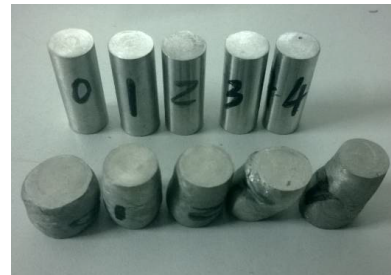
图 4 高温压缩试验前后的试样对比 Fig.4 Comparison of specimens before and after the compression test (120 °C)
