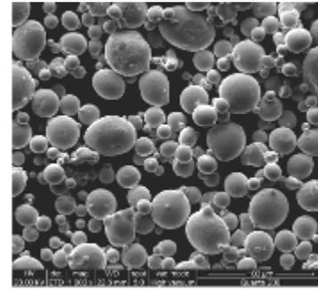
Fig.1 SEM image of CoCr-1 alloy powder
