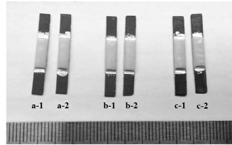
Fig.4 Three-point bending test specimens
