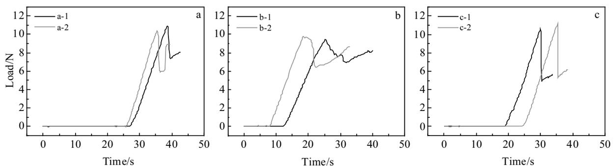
Fig.5 Time-stress curves of CoCr alloy with different surface roughness: (a) group a, (b) group b, and (c) group c
