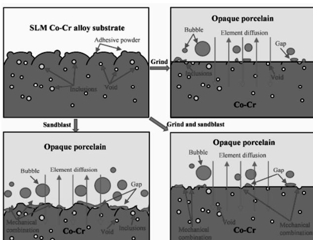
Fig.9 Influence mechanism of pretreatment process on metal-porcelain bonding properties of CoCr alloy
