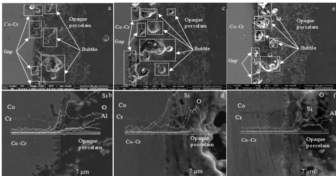
Fig.6 SEM surface morphologies (a, c, e) and EDS spectra (b, d, f) of metal-porcelain bonding interface: (a, b) group a, (c, d) group b, and (e, f) group c
