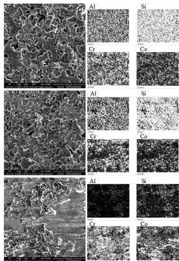
Fig.8 SEM surface morphologies and EDS maps of porcelain peeling surface: (a) group a, (b) group b, and (c) group c
