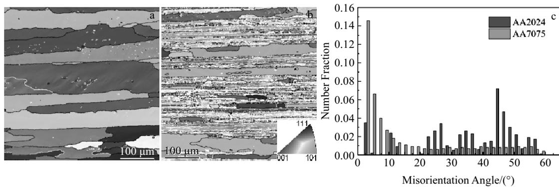
Fig.3 Grain structure of BMs: (a) AA2024, (b) AA7075, and (c) the misorientation angle distribution of the two BMs
