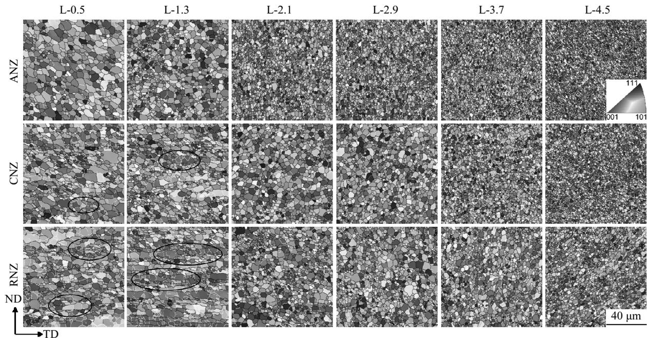
Fig.4 Grain structure variation along the weld thickness in the ANZ, CNZ, and RNZ
