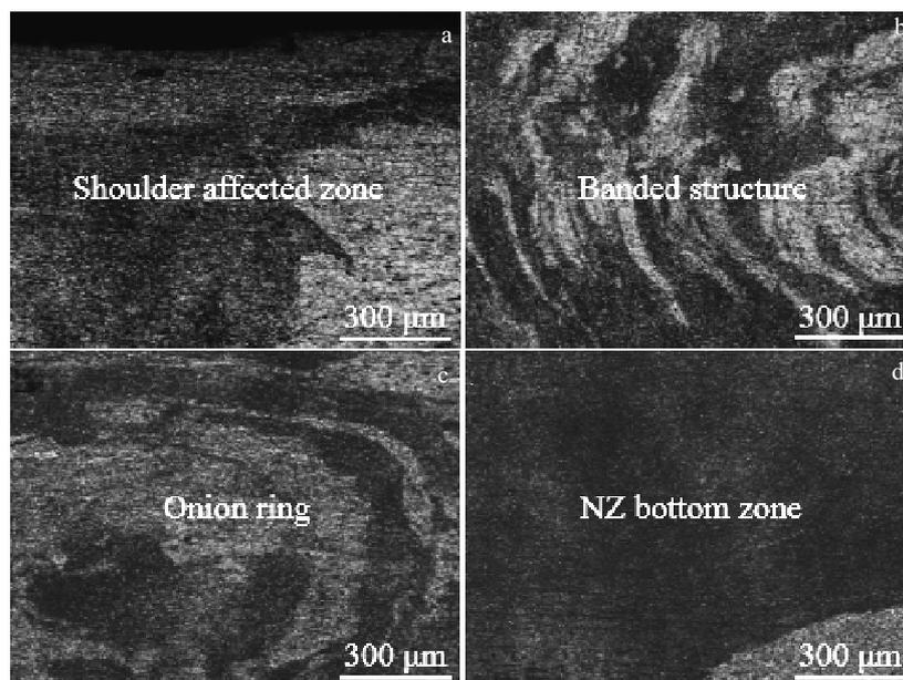
Fig.2 Metallographic structure in the top (a), the middle (b, c) and the bottom (d) of the NZ in the joint
