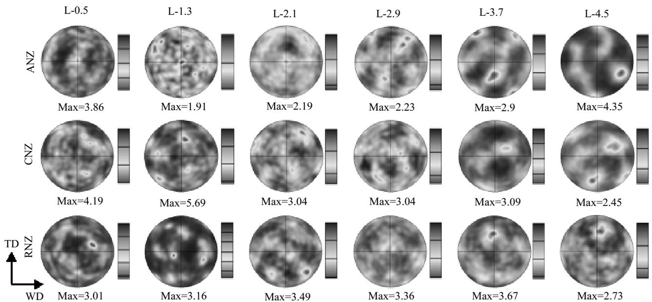
Fig.8 {111} pole figures at the different locations of the NZ along the weld thickness direction
