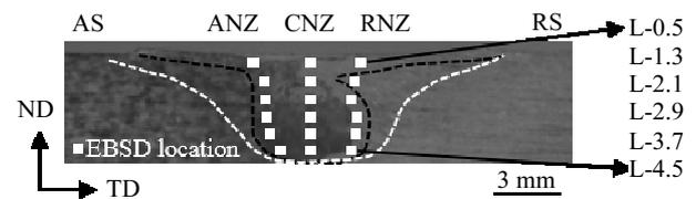
Fig.1 Macroscopic photograph of the dissimilar joint
