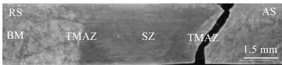
Fig.12 Cross-sectional macrostructure of FSW specimen after fatigue test
