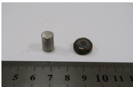
Fig.1 Photo of samples before and after hot compression test
