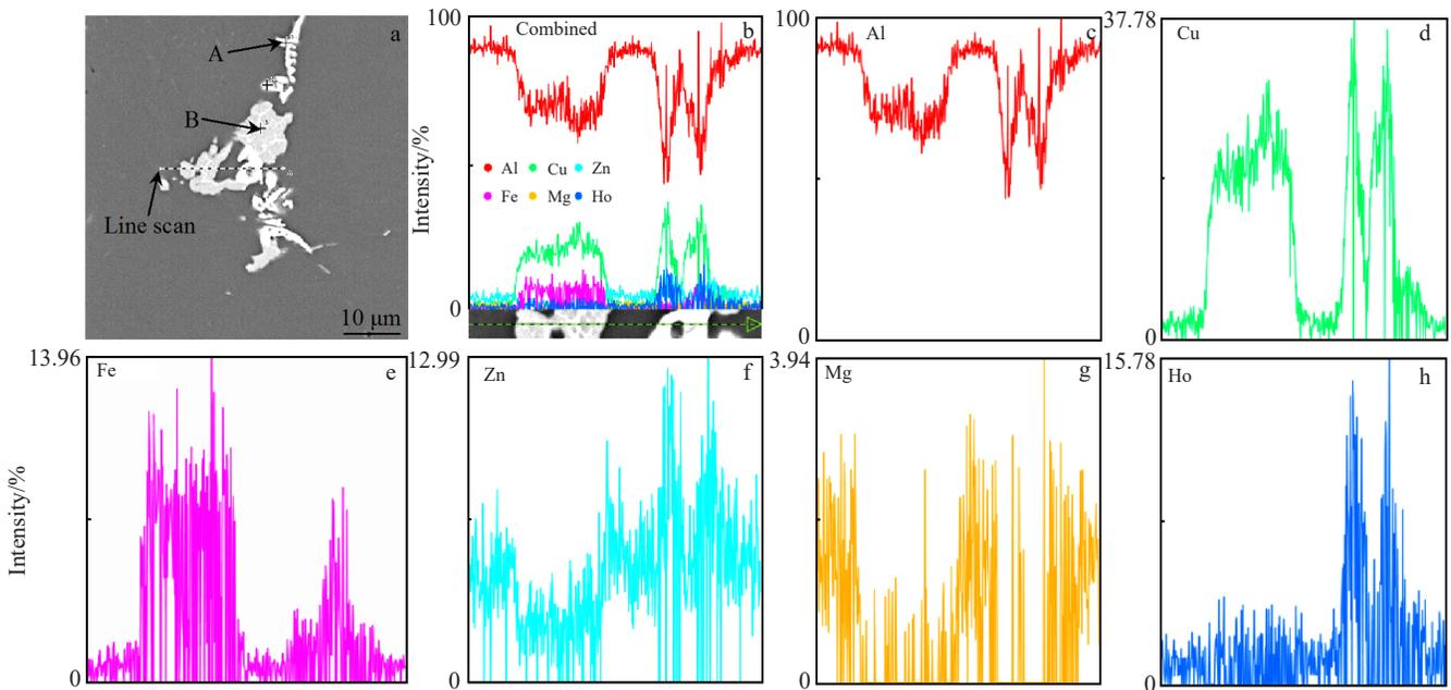
Fig.7 SEM image (a) and corresponding element distribution along marked line in Fig.7a (b-h) for homogenized alloy
