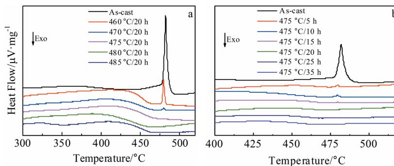
Fig.5 DSC curves of the alloy homogenized at different temperatures for 20 h (a) and for different time at 475 °C (b)
