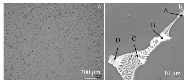
**Fig. 2** OM (a) and SEM (b) images of as-cast Al-Zn-Mg-Cu alloy with Ho addition
