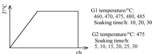
**Fig. 1** Schematic diagram of the homogenization treatment
