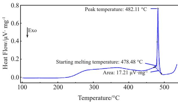
Fig.4 DSC curve of the as-cast alloy
