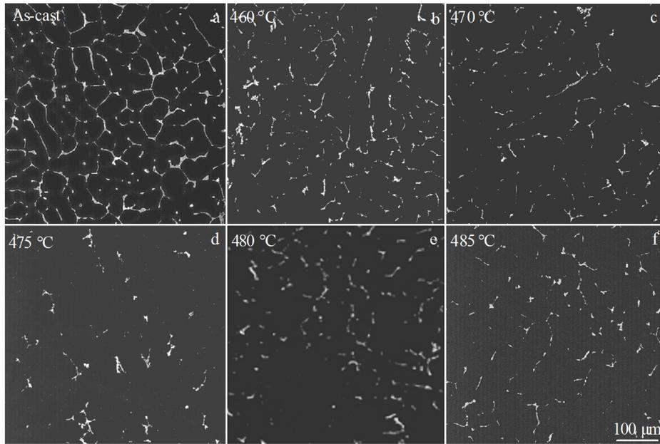
Fig.6 SEM images of second phases in as-cast alloy (a) and the alloys homogenized at different temperatures for 20 h
