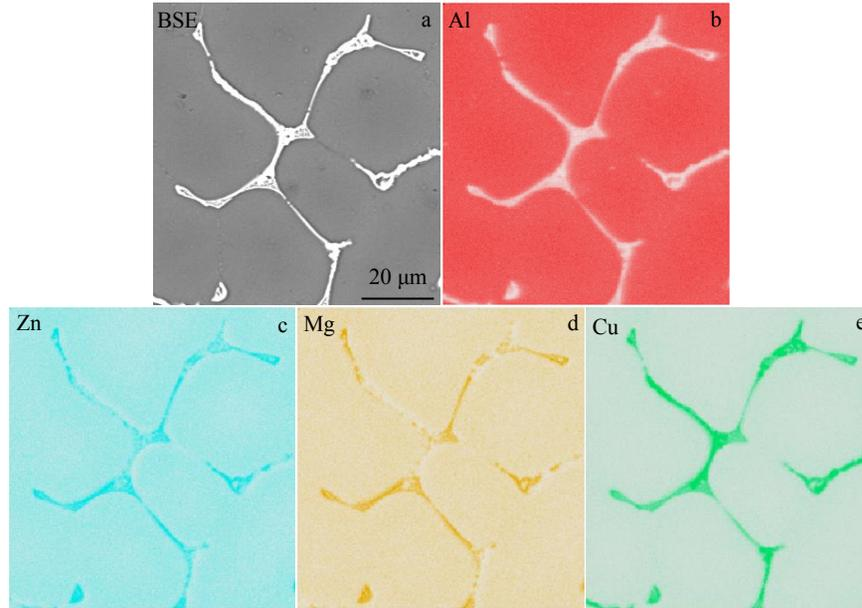
Fig.3 SEM image (a) and corresponding element distribution of Al (b), Zn (c), Mg (d), and Cu (e) of as-cast alloy
