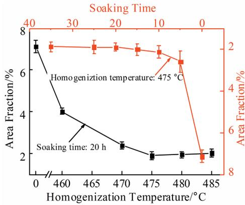
**Fig.8** Area fraction of intermetallic phases after different homogenization treatments
