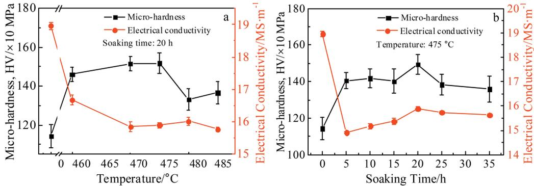
**Fig.9** Micro-hardness and electrical conductivity of homogenized alloy at different temperatures (a) for different soaking time (b)
