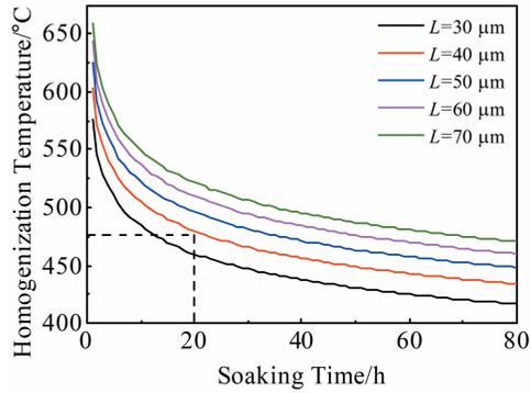
Fig.10 Homogenization kinetic curves of the alloy with different T (AlZnMgCu) phase spacing
