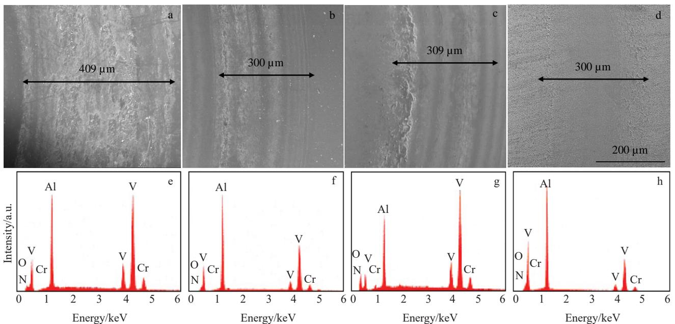
Fig.9 Wear track morphologies (a~d) and EDS spectra (e~h) of AlCrN/AlCrVN multi-layer coatings at high temperature: (a, e) AlCrN/AlCrVN-1, (b, f) AlCrN/AlCrVN-2, (c, g) AlCrN/AlCrVN-4, and (d, h) AlCrN/AlCrVN-6
