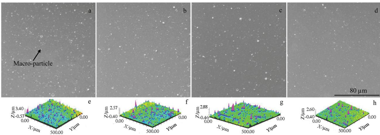
Fig.2 SEM surface morphologies (a~d) and 3D surface morphologies (e~h) of AlCrN/AlCrVN-1 (a, e), AlCrN/AlCrVN-2 (b, f), AlCrN/AlCrVN-4 (c, g), and AlCrN/AlCrVN-6 (d, h) multi-layer coatings
