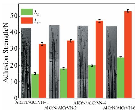
Fig.6 Scratch images and adhesion strength of AlCrN/AlCrVN multi-layer coatings
