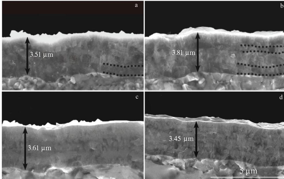
Fig.1 SEM cross-section morphologies of AlCrN/AlCrVN-1 (a), AlCrN/AlCrVN-2 (b), AlCrN/AlCrVN-4 (c), and AlCrN/AlCrVN-6 (d) multi-layer coatings
