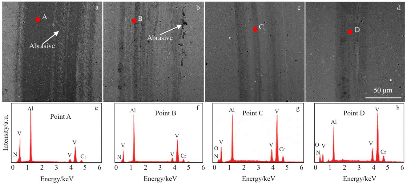
Fig.8 Wear track morphologies (a~d) and EDS spectra of red points A~D in Fig.8a~8d (e~h) of AlCrN/AlCrVN multi-layer coatings at room temperature: (a, e) AlCrN/AlCrVN-1, (b, f) AlCrN/AlCrVN-2, (c, g) AlCrN/AlCrVN-4, and (d, h) AlCrN/AlCrVN-6
