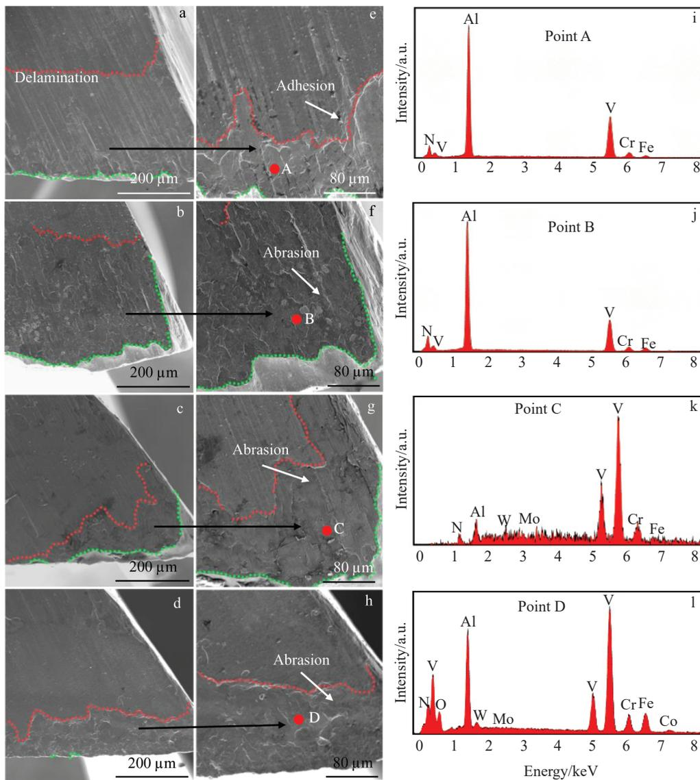
Fig.11 Flank surface morphologies (a~h) and EDS spectra of red points A~D in Fig.11e~11h (i~l) of AlCrN/AlCrVN end milling cutters: (a, e, i) AlCrN/AlCrVN-1, (b, f, j) AlCrN/AlCrVN-2, (c, g, k) AlCrN/AlCrVN-4, and (d, h, l) AlCrN/AlCrVN-6
