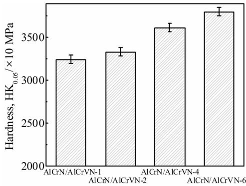
Fig.5 Hardness of AlCrN/AlCrVN multi-layer coatings
