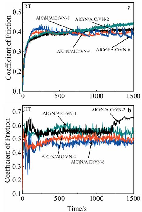
Fig.7 COF of AlCrN/AlCrVN multi-layer coatings at room temperature (a) and high temperature (b)
