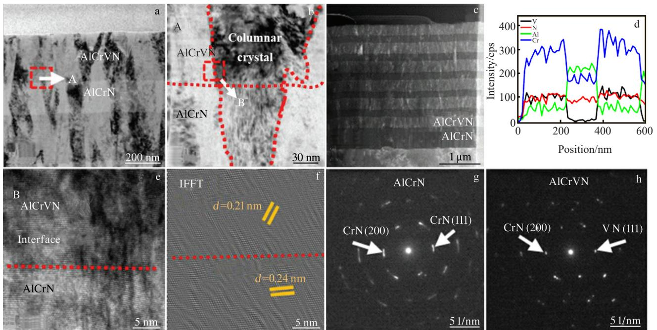
**Fig. 4** TEM cross-section morphology (a) and magnified TEM image of area A in Fig. 4a (b) of AlCrN/AlCrVN-6 multi-layer coating; TEM cross-section morphology (c) and corresponding EDS spectra (d) of AlCrN/AlCrVN-6 multi-layer coating; HRTEM image of area B in Fig. 4b (e) and corresponding IFFT image (f) of AlCrN/AlCrVN-6 multi-layer coating; SAED patterns of AlCrN layer (g) and AlCrVN layer (h)
