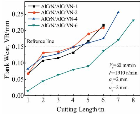
Fig.10 Cutting life curves of different AlCrN/AlCrVN end milling cutters at cutting speed of 60 m/min
