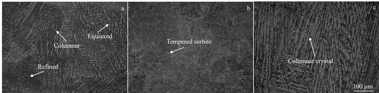
Fig.8 Metallographic microstructures of WFZ in as-received (a), tempered (b), and STA-treated (c) welding joints
