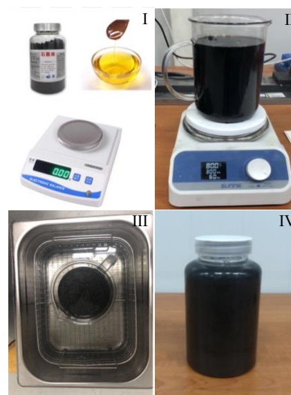
Fig.1 Preparation process of cutting nanofluid
