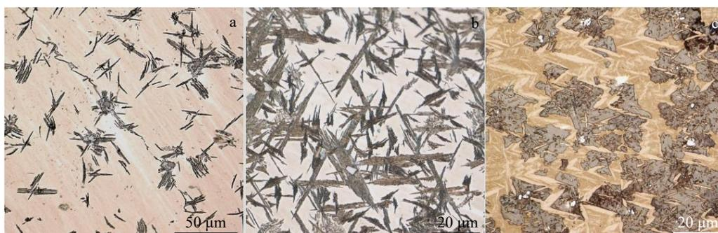
Fig.4 Typical morphologies of transformation products taken from the samples after interrupted isothermal treatment: (a) 635 °C, 20 min; (b) 600 °C, 8.5 min; (c) 500 °C, 5 min
