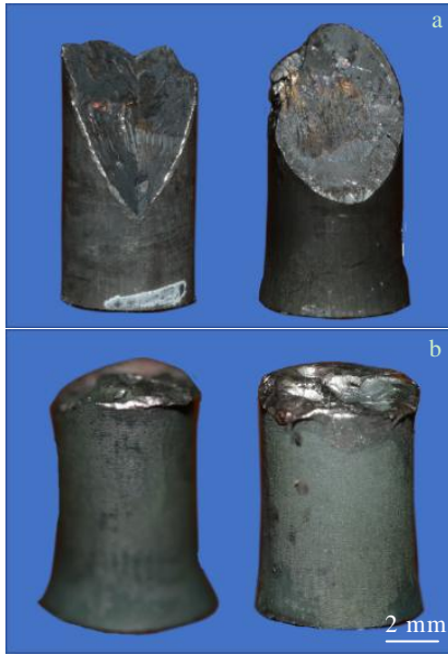
图 2 单晶高温合金 CMSX-4 低周疲劳断口宏观特征 Fig.2 Macro-morphologies of low cycle fatigue fracture of single crystal superalloy CMSX-4 at temperature of 760 °C (a) and 950 °C (b)
