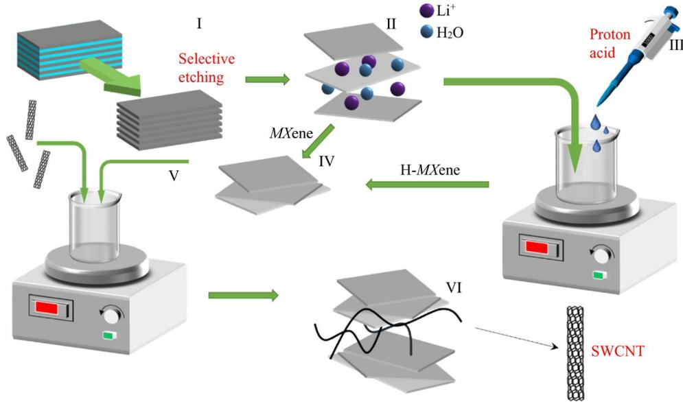
Fig.1 Schematic diagrams of preparation process of SWCNT/MXene and SWCNT/H-MXene materials
