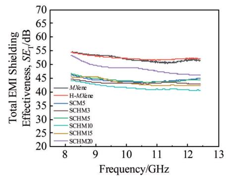
Fig.5 Total EMI shielding effectiveness of different materials
