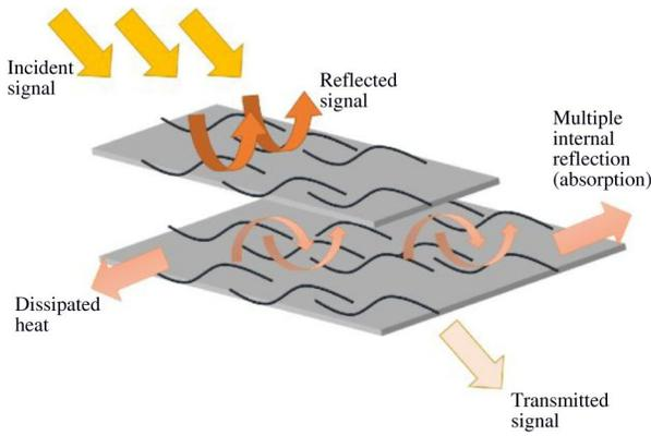
Fig.8 EMI shielding mechanism of *MXene* layer structure
