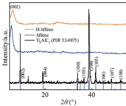
Fig.2 XRD patterns of MXene and H-MXene materials
