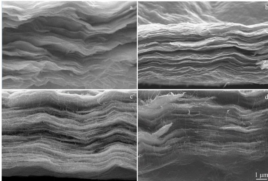
Fig.3 SEM cross-sectional morphologies of *MXene* (a), *H-MXene* (b), *SCM20* (c), and *SCHM20* (d) materials
