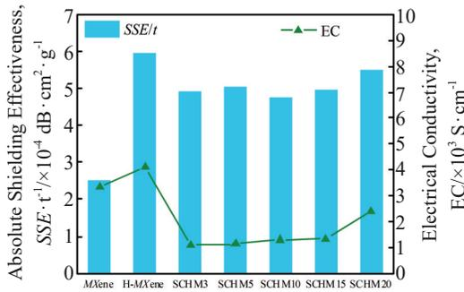
Fig.7 Absolute shielding effectiveness ( $SSE/t$ ) and electrical conductivity (EC) of different materials
