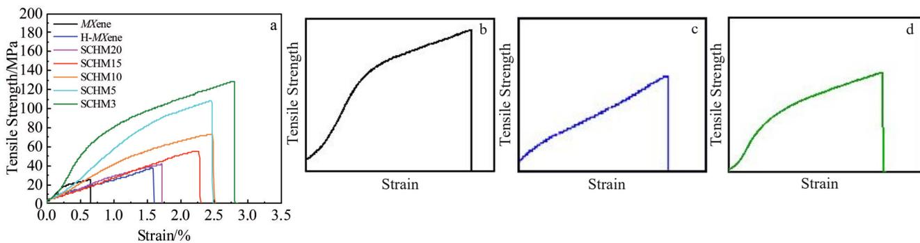
Fig.9 Tensile strength of different materials (a); schematic diagrams of tensile strength curve of *MXene* (b), H-*MXene* (c) and SCHM3 (d) materials
