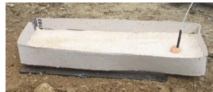
Fig.4 Appearance of experiment device of explosive welding
