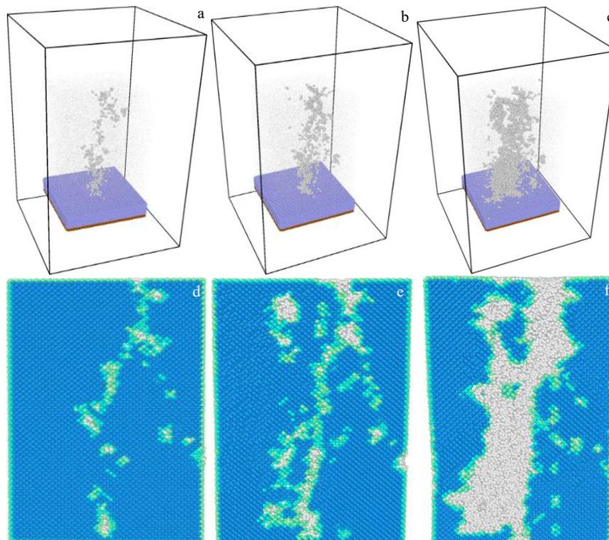
Fig.3 3D (a–c) and cross-sectional (d–f) morphologies of matrix after ion implantation with different ion doses: (a, d)  $1.0 \times 10^{13}$  ion/cm<sup>2</sup>; (b, e)  $2.5 \times 10^{13}$  ion/cm<sup>2</sup>; (c, f)  $6.25 \times 10^{13}$  ion/cm<sup>2</sup>
