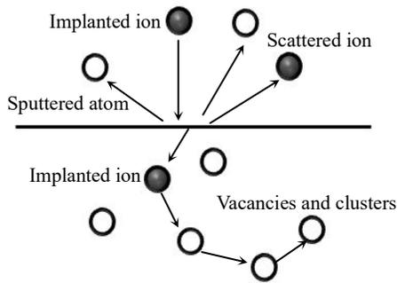
Fig.2 Interaction between implanted ions and matrix
