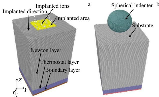
Fig.1 Schematic diagrams of 3D simulation models of ion implantation (a) and nano-indentation (b)
