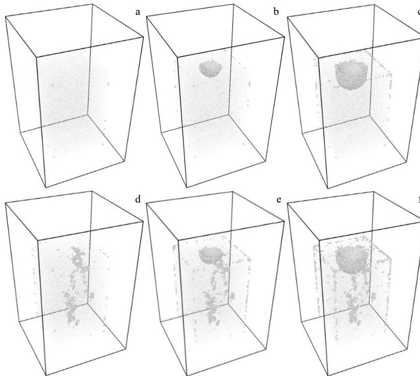
Fig.4 Morphologies of unmodified (a–c) and modified (d–f) Ge during nano-indentation simulation under ion dose of  $1.0 \times 10^{13}$  ion/cm<sup>2</sup>: (a, d) initial damage; (b, e) damage propagation; (c, f) final damage
