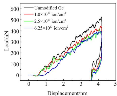
Fig.5 Load-displacement curves of nano-indentation process under different ion doses
