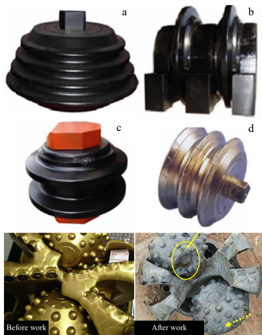
图 1 典型的盾构机刀具以及工作前和工作 80 h 后钻头对比 Fig.1 Comparison of typical shield machine [21,25] : (a) positive roller cutter, (b) double center cutter, (c) double-edged roller cutter, (d) three-flute roller cutter with tungsten carbide; (e) drill bit before work, and (f) drill bit after 80 h working
