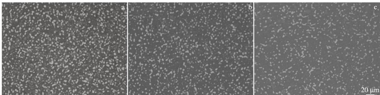
Fig.3 Microstructures of Ti555211 titanium alloy after treatments at different solution temperatures: (a) 780 °C/2 h/AC+600 °C/9 h/AC; (b) 800 °C/2 h/AC+600 °C/12 h/AC; (c) 820 °C/2 h/AC+600 °C/6 h/AC
