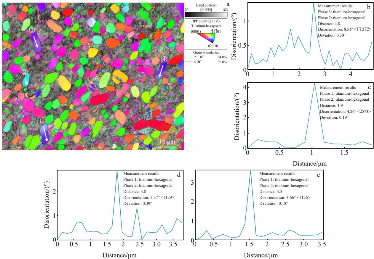
Fig.8 IPF orientation of  $\alpha$  phase in Ti555211 titanium alloy (a); internal orientations of  $\alpha$  phase along arrow 1 (b), arrow 2 (c), arrow 3 (d), and arrow 4 (e) in Fig.8a
