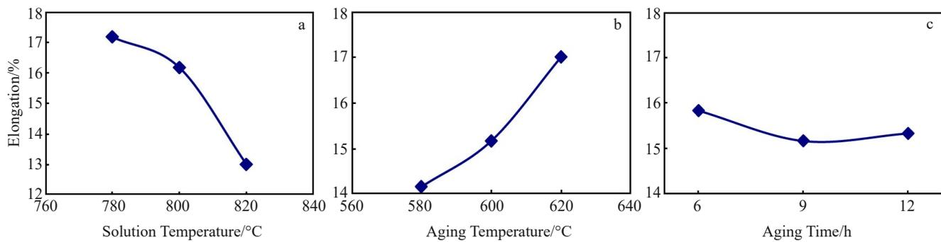
Fig.2 Relationships of elongation with solution temperature (a), aging temperature (b), and aging time (c)
