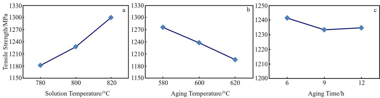
Fig.1 Relationships of tensile strength with solution temperature (a), aging temperature (b), and aging time (c)
