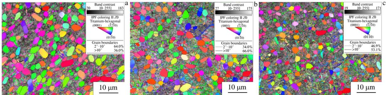
Fig.7 IPF orientations of Ti555211 titanium alloys after different treatments: (a) 780 °C/2 h/AC+620 °C/12 h/AC; (b) 800 °C/2 h/AC+600 °C/12 h/AC; (c) 820 °C/2 h/AC+580 °C/12 h/AC
