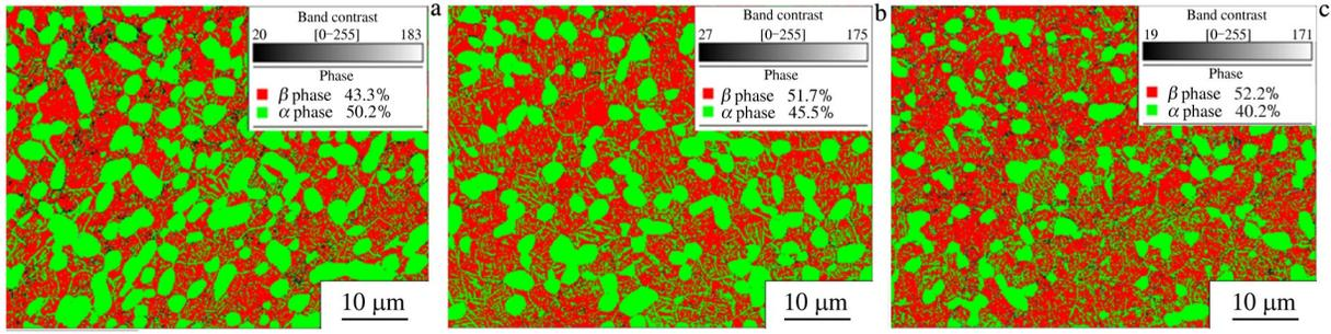
Fig.6 Phase distributions of Ti555211 titanium alloys after different treatments: (a) 780 °C/2 h/AC+620 °C/12 h/AC; (b) 800 °C/2 h/AC+600 °C/12 h/AC; (c) 820 °C/2 h/AC+580 °C/12 h/AC
