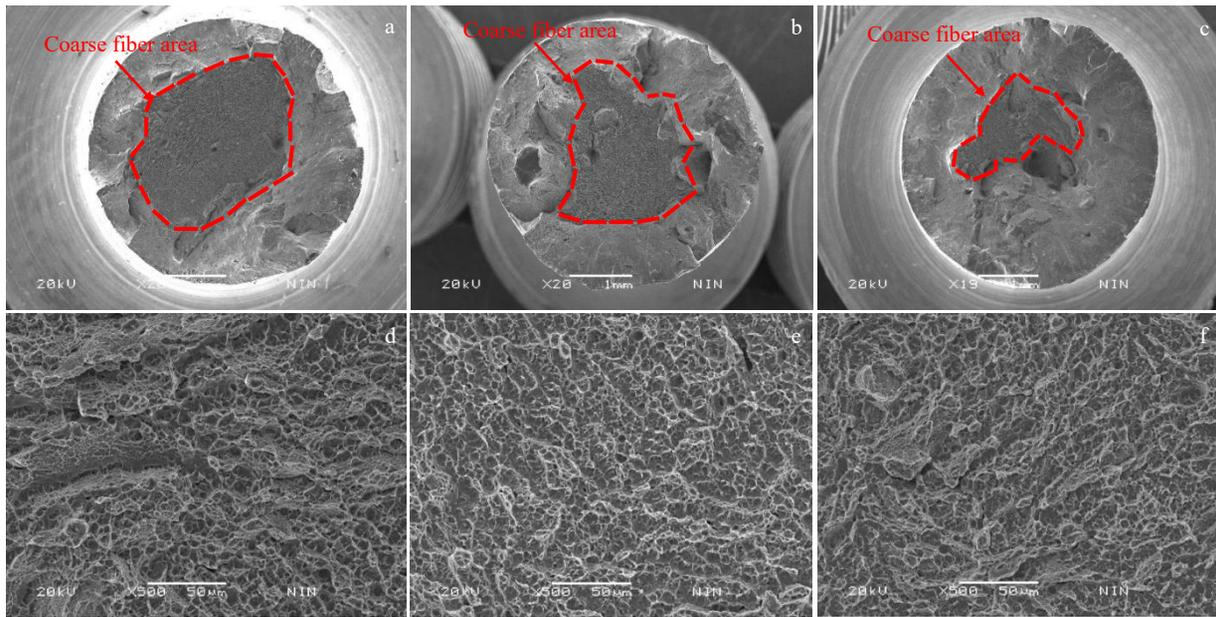
Fig.5 Room temperature tensile fracture morphologies of Ti555211 titanium alloy bars after treatments at different solution temperatures: (a, d) 780 °C/2 h/AC+600 °C/9 h/AC; (b, e) 800 °C/2 h/AC+600 °C/12 h/AC; (c, f) 820 °C/2 h/AC+600 °C/6 h/AC
