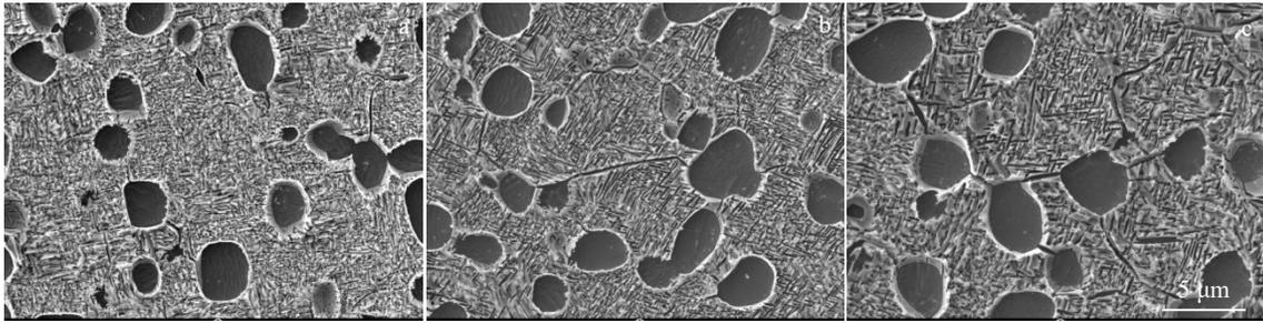
Fig.4 Microstructures of Ti555211 titanium alloy after treatments at different aging temperatures: (a) 820 °C/2 h/AC+580 °C/6 h/AC; (b) 820 °C/2 h/AC+600 °C/9 h/AC; (c) 820 °C/2 h/AC+620 °C/12 h/AC
