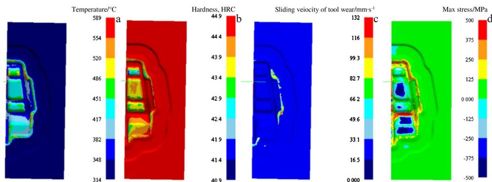
Fig. 8 Temperature (a), hardness (b), sliding velocity (c), and max principal stress (d) of forging die
