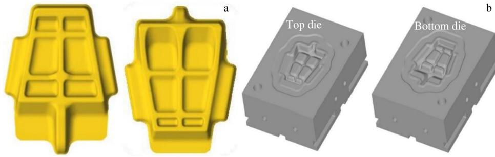
Fig.4 Schemes of forging (a) and dies (b)
