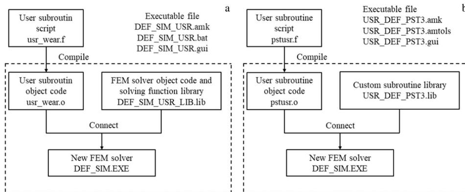
Fig.2 Schematic diagrams of secondary development: (a) pre-process and (b) post-process
