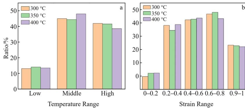
Fig.11 Ratio of temperature range (a) and strain range (b) at different die temperatures
