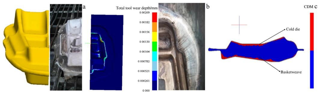
Fig. 7 Comparison between forging experiment and simulation: (a) forging shape, (b) wear distribution, and (c) macrostructure delamination of forging
