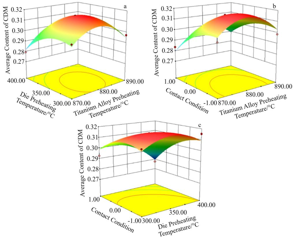
Fig.10 3D surface plots of average CDM content in different interaction conditions: (a) different die and titanium alloy preheating temperatures, (b) different titanium alloy preheating temperatures and contacting conditions, and (c) different die preheating temperatures and contacting conditions
