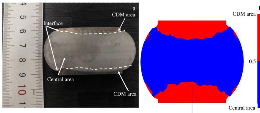
Fig.3 Comparison of forging test (a) and simulation (b) results
