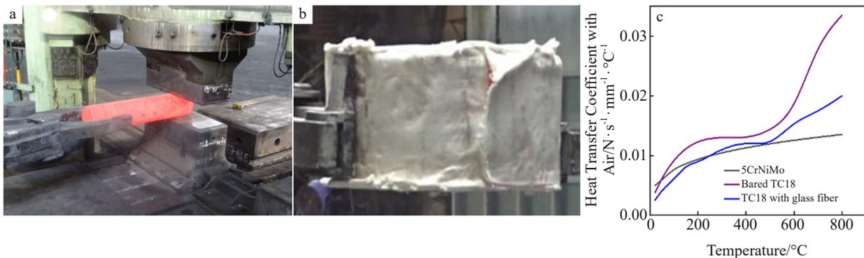
Fig.6 Bare metal (a), metal with glass fiber (b), and heat transfer coefficient (c)
