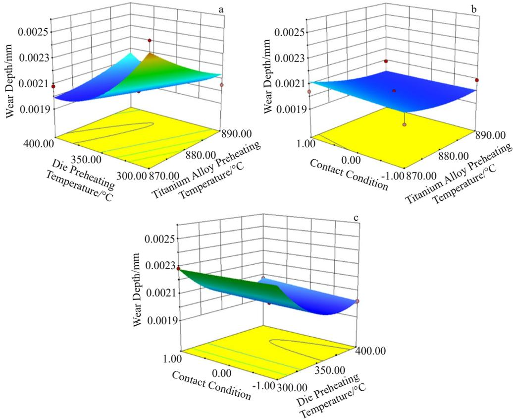
Fig.12 3D surface plots of wear depth at different conditions: (a) varying die and titanium alloy preheating temperatures, (b) varying titanium alloy preheating temperatures and contacting conditions, and (c) varying die preheating temperatures and contacting conditions
