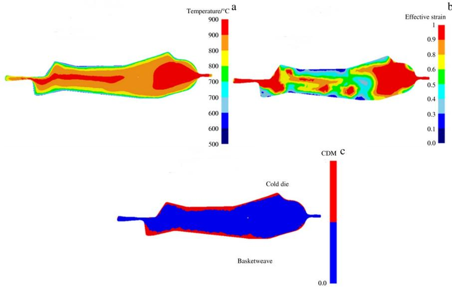
Fig.9 Temperature field (a), strain field (b), and macrostructure delamination (c) of forging
