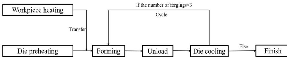
Fig.5 Scheme of the simulation
