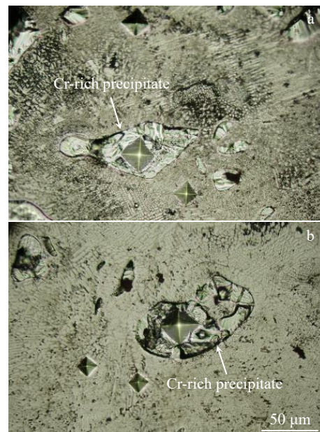
Fig. 7 Vickers hardness indentation morphologies of Ni-60Cr (a) and Ni-80Cr (b)
