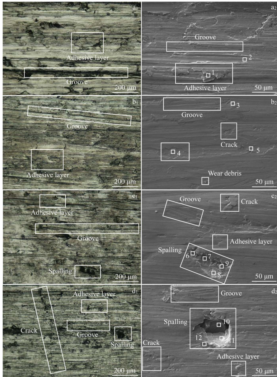
Fig.9 Surface morphologies of Ni-20Cr (a 1 -a 2 ), Ni-40Cr (b 1 -b 2 ), Ni-60Cr (c 1 -c 2 ), and Ni-80Cr (d 1 -d 2 ) after wear test
