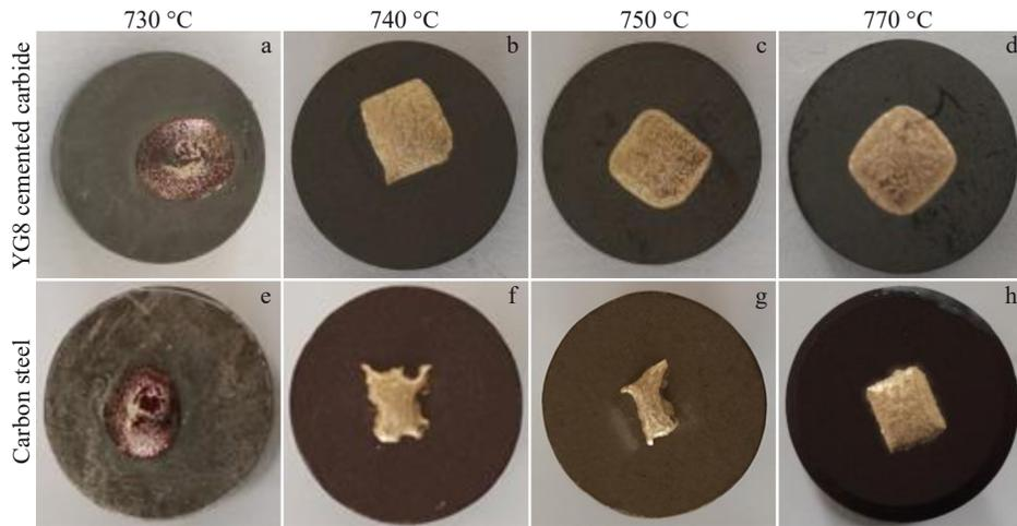
Fig.2 Spread morphologies of joints at YG8 cemented carbide side (a–d) and carbon steel side (e–h) brazed at different temperatures after wettability test: (a, e) 730 °C; (b, f) 740 °C; (c, g) 750 °C; (d, h) 770 °C
