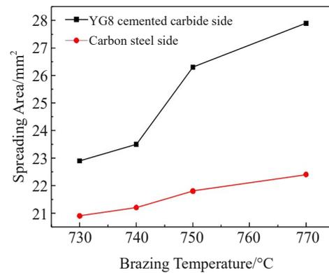
Fig.4 Spreading area of joints brazed at different temperatures
