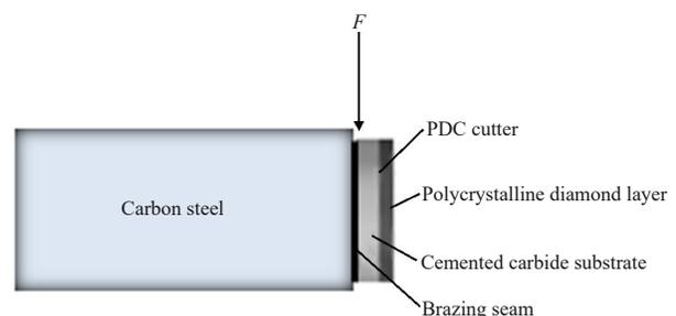
Fig.1 Schematic diagram of shear test for brazing joint
