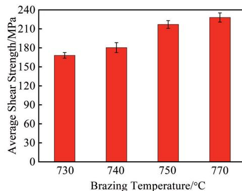
Fig.5 Average shear strength of joints brazed at different temperatures
