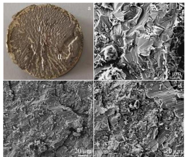
Fig.9 Fracture morphologies of joints brazed at 730 °C: (a) appearance, (b) magnified image of region I, and (c–d) magnified images of region II marked in Fig.9a
