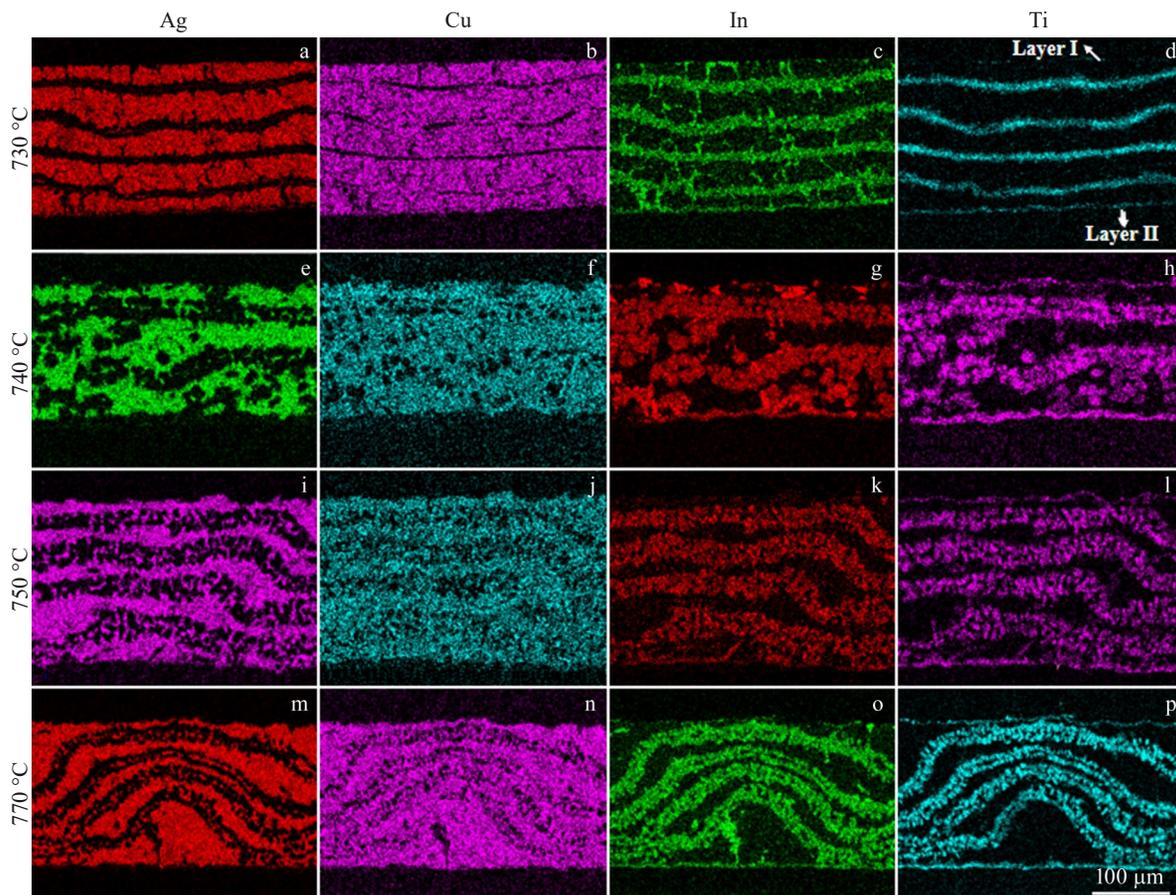
Fig.7 Element distributions of Ag (a, e, i, m), Cu (b, f, j, n), In (c, g, k, o), and Ti (d, h, l, p) across interface of joints brazed at different temperatures: (a–d) 730 °C, (e–h) 740 °C, (i–l) 750 °C, and (m–p) 770 °C
