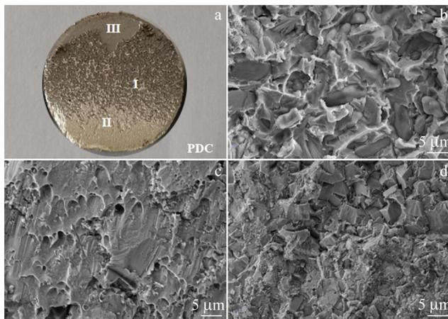
Fig.10 Fracture morphologies of joints brazed at 770 °C: (a) appearance, (b) magnified image of region I, (c) magnified image of region II, and (d) magnified image of region III marked in Fig.10a
