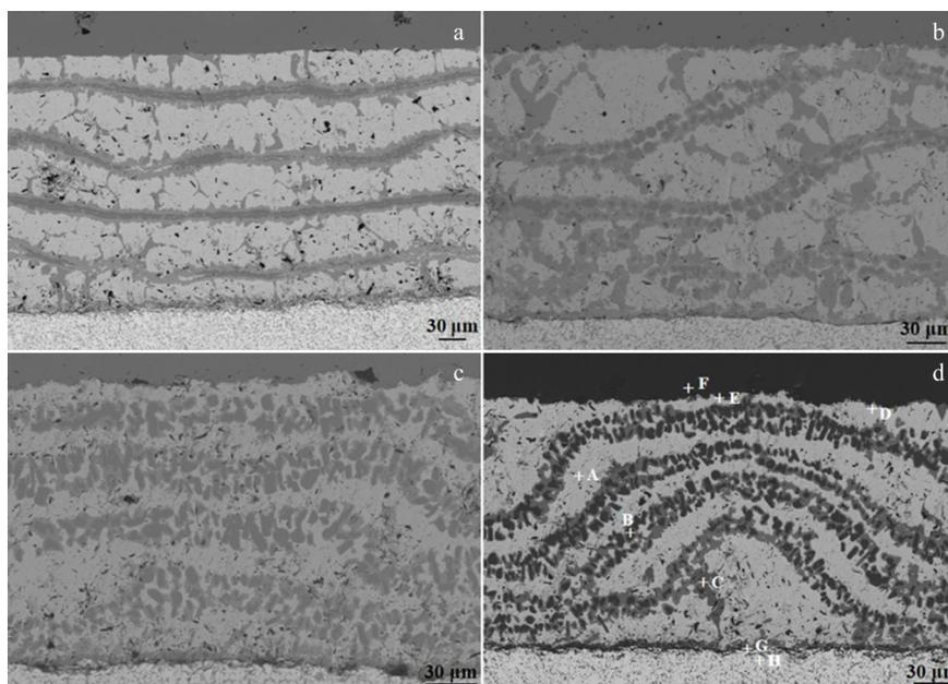
Fig.6 Interfacial microstructures of joints brazed at different temperatures: (a) 730 °C, (b) 740 °C, (c) 750 °C, and (d) 770 °C
