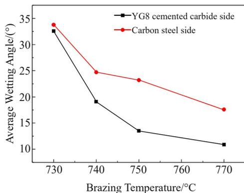
Fig.3 Average wetting angle of joints brazed at different temperatures
