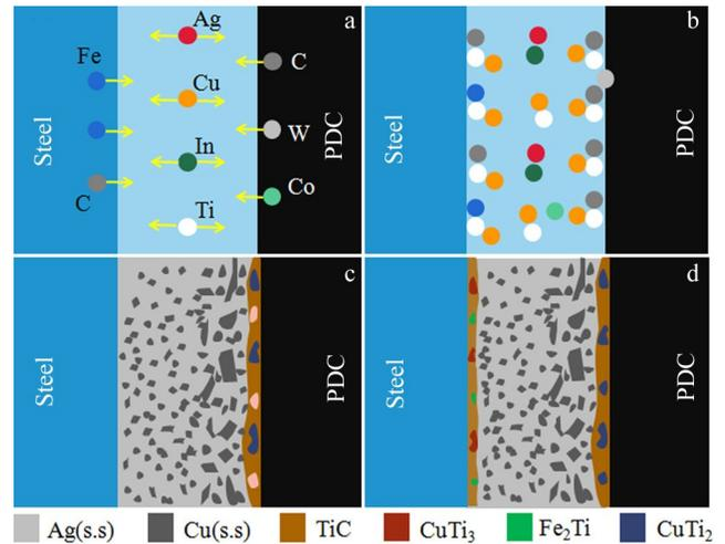
Fig.8 Schematic diagrams of microstructure evolution of joint between PDC cutters and carbon steel
