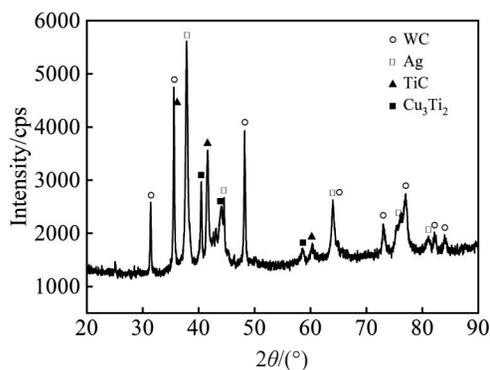
Fig.11 XRD pattern of fracture surface of joint brazed at 770 °C
