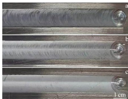
Fig.4 Surface morphologies of Al-Li/Ti friction stir lap welded joints under 800-60 condition (a), 800-120 condition (b), and 1000-240 condition (c)
