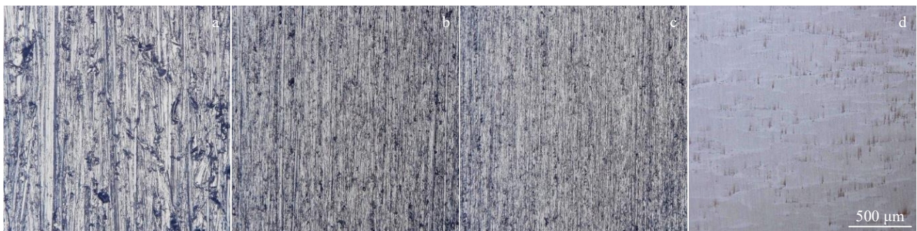
Fig.1 Surface morphologies of 80-grit (a), 400-grit (b), 1200-grit (c), and polished (d) samples
