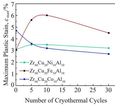
Fig.2 Relationship between maximum plastic strain  $\varepsilon_{\max}$  and the number of cryothermal cycles for different MGs<sup>[33]</sup>
