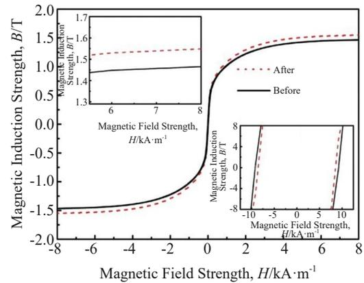
Fig.3 Magnetization property curves of melt-spun  $\text{Fe}_{80}\text{Si}_{8.75}\text{B}_{10}\text{Cu}_{1.25}$  MG ribbons before and after thermal cycling<sup>[42]</sup>
