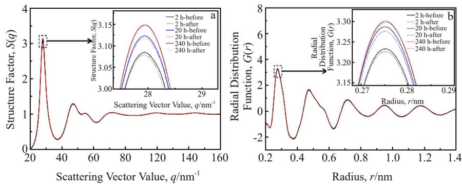
Fig.6 Structure factor (a) and reduced radial distribution function (b) of  $Zr_{46}Cu_{38}Al_8Ag_8$  MG before and after thermal cycling for different durations<sup>[35]</sup>
