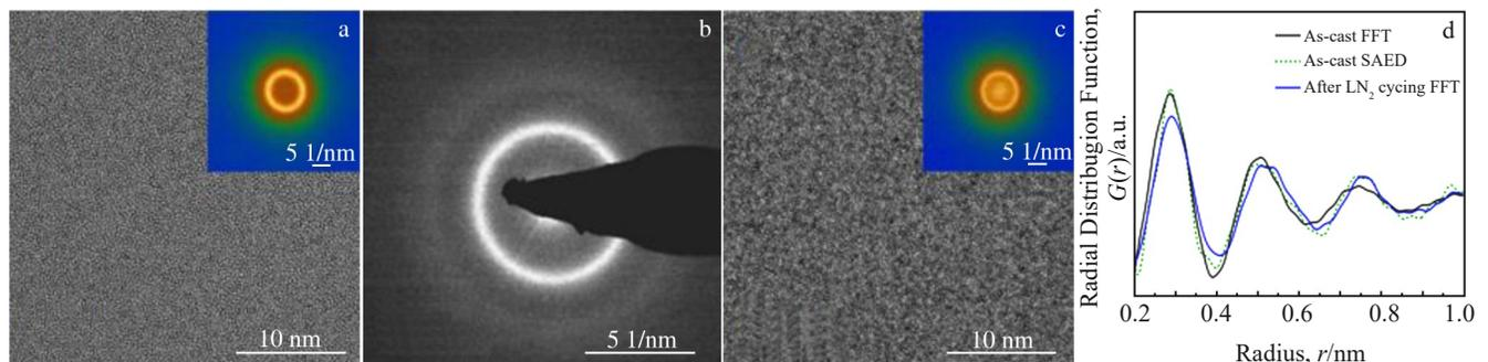
Fig. 4 HRTEM images of as-cast  $Zr_{60}Ni_{20}Fe_{10}Al_{10}$  BMG before (a) and after (c) 10 cryothermal cycles with corresponding FFT patterns; SAED pattern corresponding to Fig. 4a (b); radial distribution functions derived from SAED and FFT patterns (d)<sup>[33]</sup>
