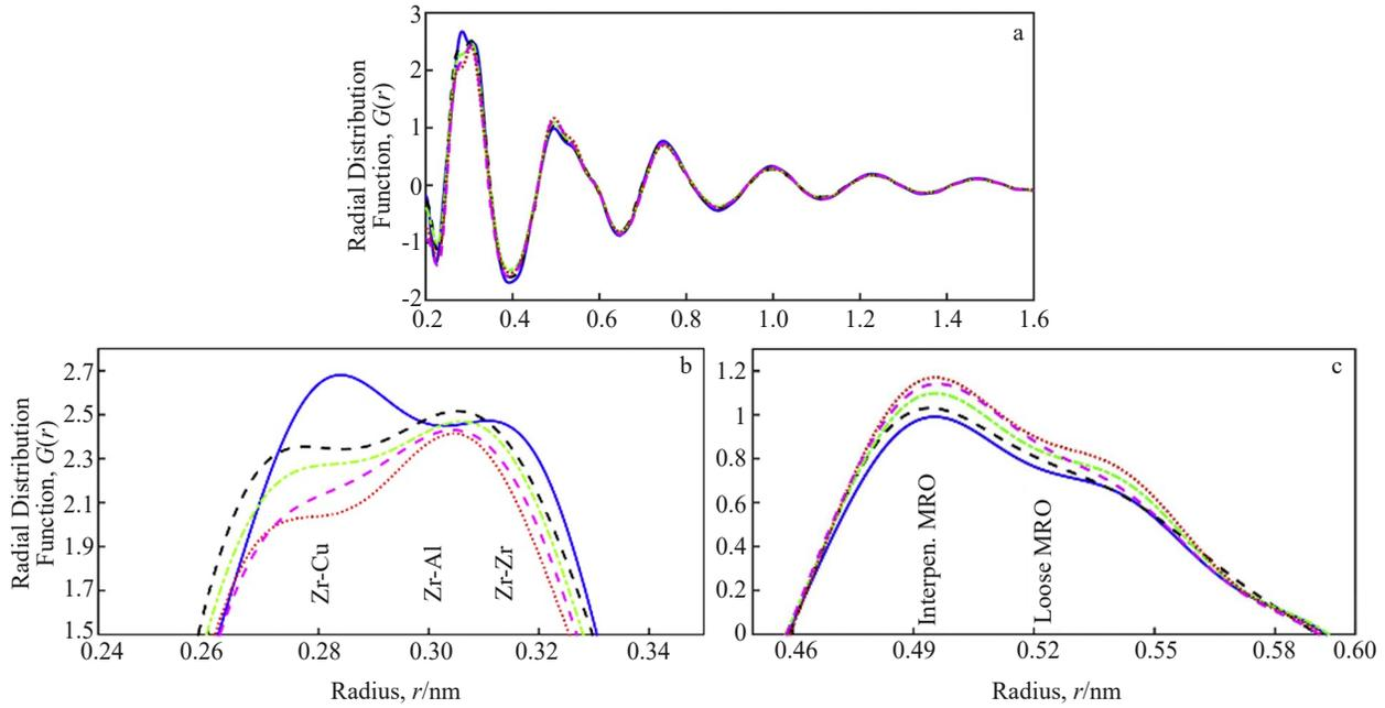
Fig.5 Comparison of radial distribution functions derived from synchrotron XRD results of  $Zr_{55}Cu_{30}Al_{10}Ni_5$  BMG after cryothermal treatment for different durations (a); enlarged images of SRO peak (b) and the first MRO peak (c) in Fig.5a<sup>[21]</sup>
