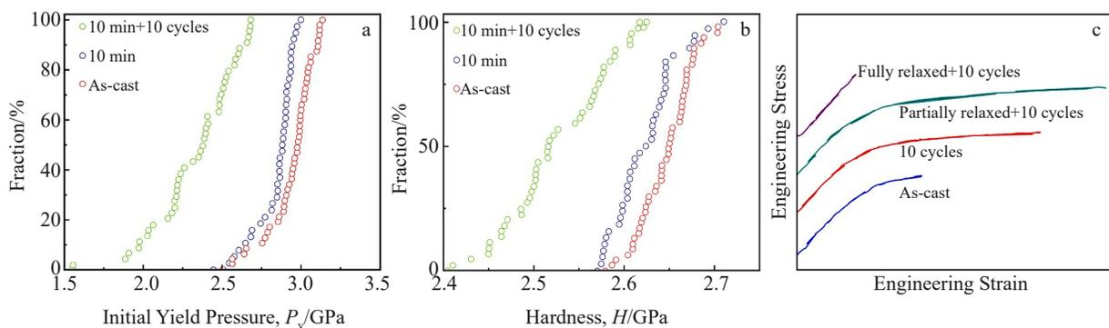
Fig.1 Statistic analysis results of initial yield pressure  $P_y$  (a) and hardness  $H$  (b) of La<sub>55</sub>Ni<sub>20</sub>Al<sub>25</sub> MG ribbon; engineering stress-engineering strain curves of Cu<sub>46</sub>Zr<sub>46</sub>Al<sub>7</sub>Gd<sub>1</sub> BMG after different treatments under uniaxial compression (c)<sup>[29]</sup>
