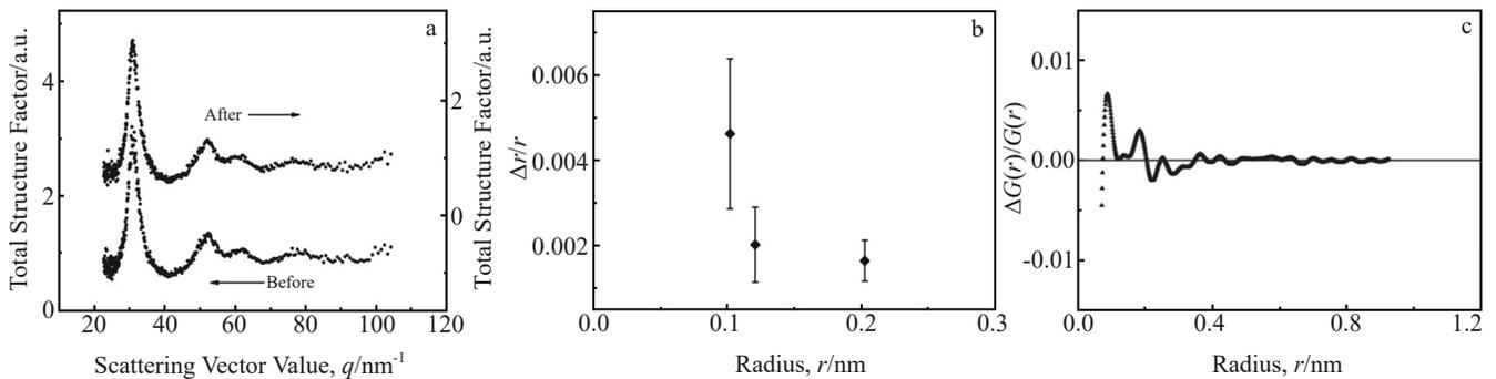
Fig.7 Total structure factor of  $Fe_{78}Cu_1Nb_4B_{3.5}Si_{13.5}$  MG before and after CT for 3 h (a); relative change of interatomic spacing after CT for 3 h (b); relative difference of total radial correlation functions of samples before and after CT for 3 h (c)<sup>[41]</sup>
