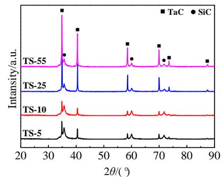
Fig.5 XRD patterns of ceramics derived from TS-5, TS-10, TS-25 and TS-55 hybrid precursors at 1873 K
