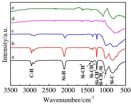
Fig.3 FTIR spectra of original PCS (a), TS-25 (b) and TS-25 precursor heat-treated at different temperatures: (c) 873 K, (d) 1073 K, and (e) 1673 K
