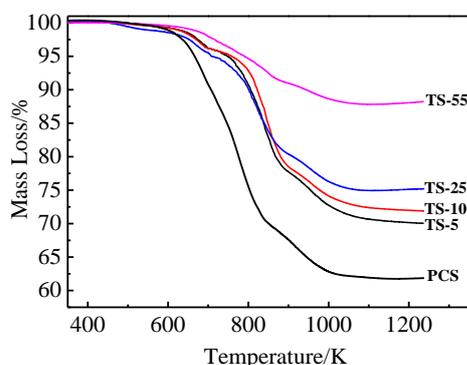
Fig.2 TGA curves of PCS and TS precursors in flowing nitrogen
