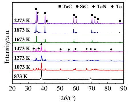
Fig.4 XRD patterns of ceramics derived from TS-25 at different temperatures
