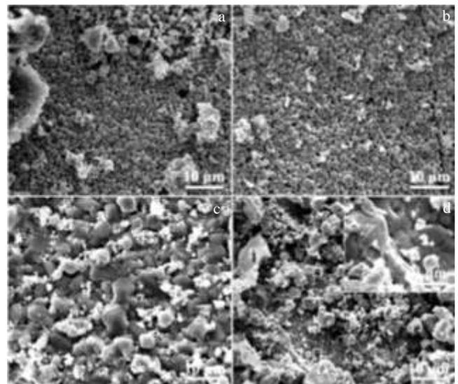
Fig.6 SEM images of ceramics derived from TS-5 (a), TS-10 (b), TS-25 (c) and TS-55 (d) hybrid precursors at 2273 K
