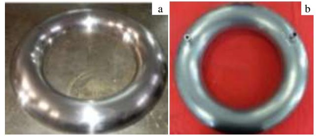
图 13 采用正反胀形方法制造的 TC4 半环及环形气瓶产品 Fig.13 TC4 semi-annular part and annular gas tank developed by direct-reverse SPF process
