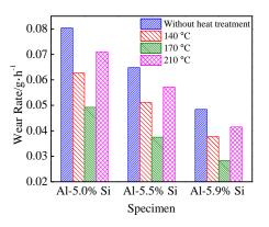
Fig.3 Wear rate of the surfacing layers welded by 4043 welding wires after different heat treatments
