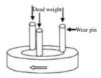
Fig.1 Schematic diagram of wear testing
