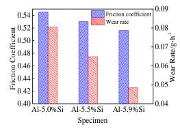
Fig.2 Wear rates and friction coefficients of the surfacing layers
