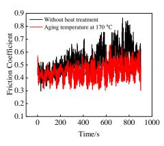
Fig.4 Friction coefficients of the surfacing layers welded with Al-5.9% Si welding wire before and after heat treatments
