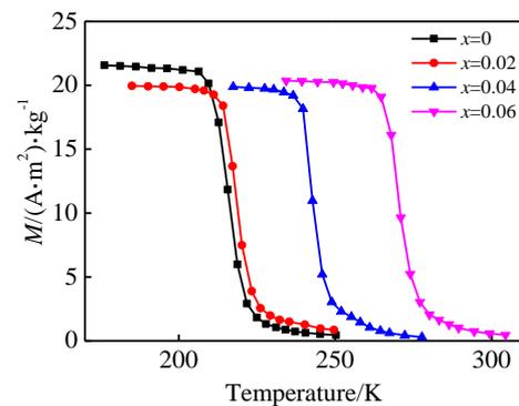
Fig.3 Temperature dependence of magnetization for La(Fe<sub>1-x</sub>Co<sub>x</sub>)<sub>11.2</sub>Si<sub>1.8</sub> ( $x=0, 0.02, 0.04, 0.06$ ) measured under a field of 0.05 T
