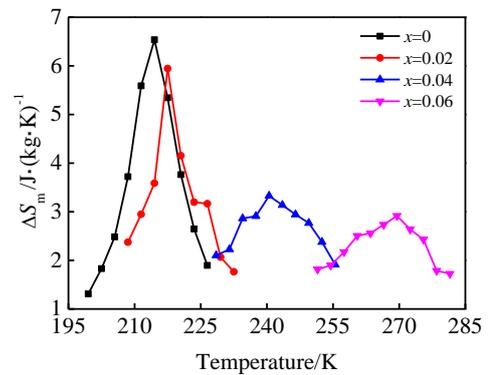
Fig.6 Magnetic entropy change  $\Delta S_m$  as functions of temperature for  $\text{La}(\text{Fe}_{1-x}\text{Co}_x)_{11.2}\text{Si}_{1.8}$  ( $x=0, 0.02, 0.04, 0.06$ ) compounds under a magnetic field change of 0~1.5 T
