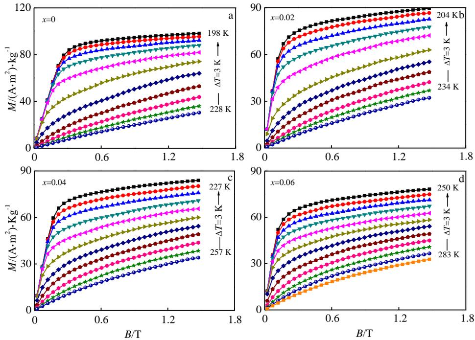
Fig.4 Magnetization isotherms of  $\text{La}(\text{Fe}_{1-x}\text{Co}_x)_{11.2}\text{Si}_{1.8}$  ( $x=0, 0.02, 0.04, 0.06$ ) measured in the vicinity of  $T_C$ : (a)  $x=0$ , (b)  $x=0.02$ , (c)  $x=0.04$ , and (d)  $x=0.06$
