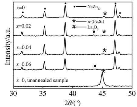
Fig.2 XRD patterns of La(Fe<sub>1-x</sub>Co<sub>x</sub>)<sub>11.2</sub>Si<sub>1.8</sub> ( $x=0, 0.02, 0.04, 0.06$ ) annealed and unannealed
