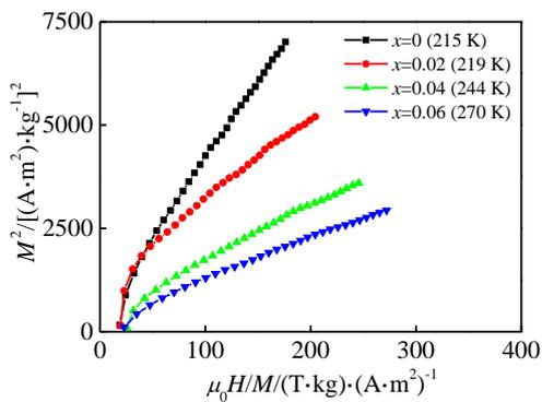
Fig.5 Arrott plots of  $\text{La}(\text{Fe}_{1-x}\text{Co}_x)_{11.2}\text{Si}_{1.8}$  ( $x=0, 0.02, 0.04, 0.06$ )
