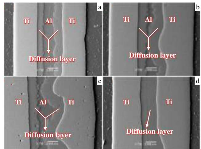
Fig.6 SEM images of Ti/Al/Ti laminates after hot pressing at 650  $^{\circ}\text{C}$  for different time: (a) 1 h, (b) 1.5 h, (c) 2 h, and (d) 2.5 h
