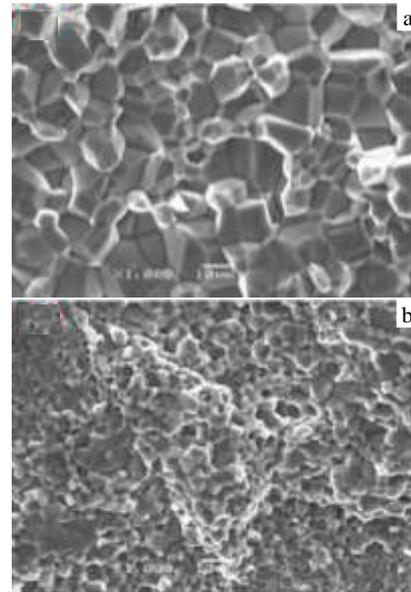
Fig.9 Fracture morphologies of diffusion layer after hot pressing for 2.5 h (a) and 3 h (b)
