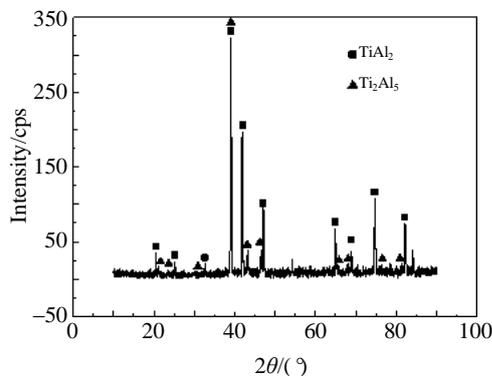
Fig.8 XRD pattern of Ti/Al/Ti laminates after hot pressing for 2.5 h
