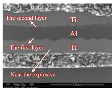
Fig.2 Bonding interface of Ti/Al/Ti laminate composites
