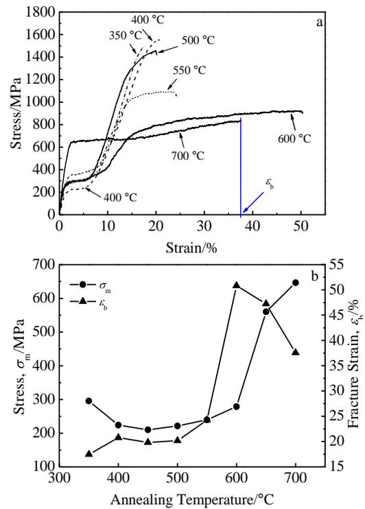
Fig.4 Effect of annealing temperature on stress-strain (a), platform stress  $\sigma_m$  and fracture strain  $\varepsilon_b$  (b) of Ti-51.1Ni alloy (test temperature 10 °C)
