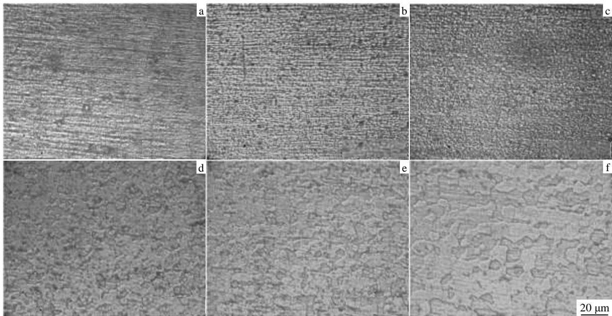
Fig.1 OM microstructures of Ti-51.1Ni alloys annealed at different temperatures: (a) 400 °C, (b) 570 °C, (c) 590 °C, (d) 600 °C, (e) 630 °C, and (f) 650 °C
