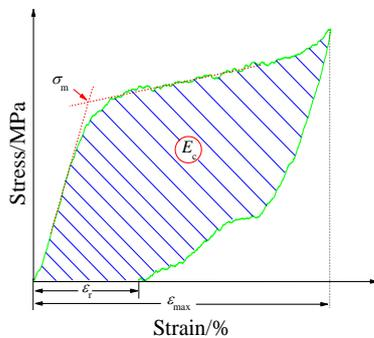
Fig.3 Definition of characteristic parameters  $\sigma_m$ ,  $\varepsilon_r$ ,  $\varepsilon_{max}$  and  $E_c$  in typical stress-strain curve ( $\sigma_m$ : platform-stress,  $\varepsilon_r$ : residual strain,  $\varepsilon_{max}$ : setting-strain value,  $E_c$ : energy consumption, i.e., the integral value of envelope area with stress-strain curve and the x axis)
