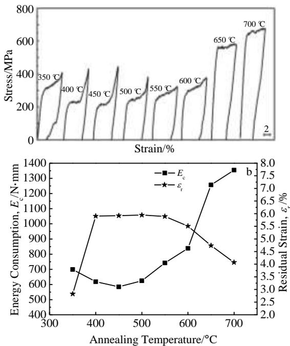
Fig.5 Effect of annealing temperature on shape memory effect, super-elasticity (a), energy consumption properties  $E_c$  and residual strain  $\epsilon_r$  (b) of Ti-51.1Ni alloy (test temperature 10 °C)
