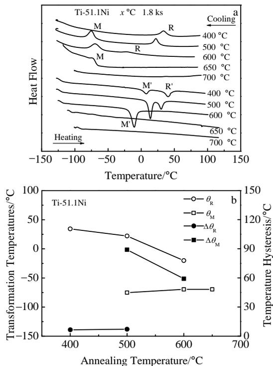
Fig.2 Effect of annealing temperature on DSC curves (a) and transformation temperatures ( $\theta_R$ ,  $\theta_M$ ), temperature hysteresis ( $\Delta\theta_M$ ,  $\Delta\theta_R$ ) (b) of Ti-51.1Ni alloy
