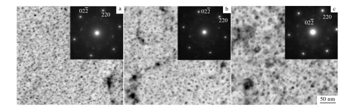
Fig.4 TEM micrographs and corresponding SAED patterns of the pre-retrogressed alloy under the external stress of 180 MPa and the stress-aging time of 4 h (a), 12 h (b), and 20 h (c)
