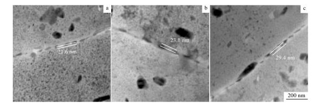
Fig.7 TEM micrographs of the retrogressed alloy under the stress-aging time of 20 h and the external stresses of 90 MPa (a), 270 MPa (b), and 0 MPa (c)
