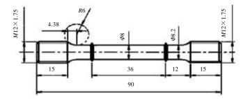
Fig.2 Geometry and size of sample (mm)
