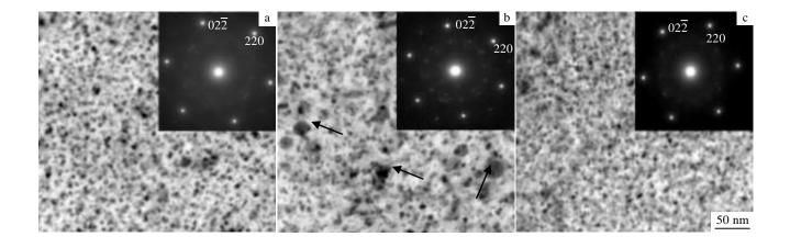
Fig.5 TEM micrographs and corresponding SAED patterns of the retrogressed alloy under the stress-aging time of 20 h and the external stresses of 90 MPa (a), 270 MPa (b), and 0 MPa (c)
