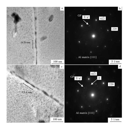
Fig.3 TEM micrographs (a, c) and corresponding SAED patterns (b, d) from <111>Al projection of the studied alloy before and after retrogression heat treatment: (a, b) T651 state, as-received material; (c, d) RHT state, 20 min heat treatment at 180 °C
