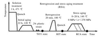
Fig.1 Retrogression and stress-aging treatment procedures
