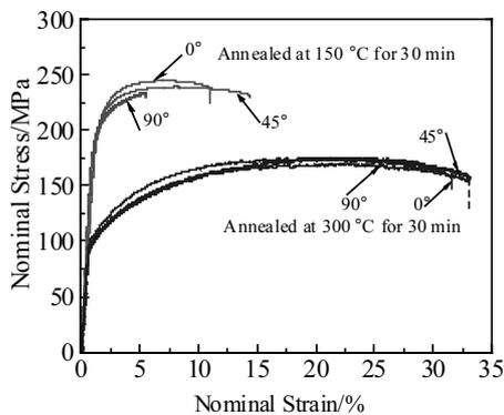
Fig.2 Nominal stress-strain curves in the tensile direction of RD, 45°, and TD of the sheets annealed at 150 and 300 °C for 30 min
