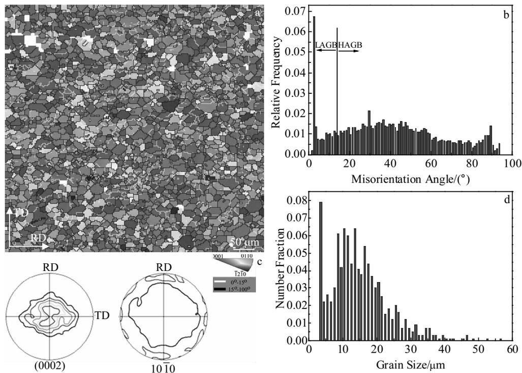
Fig.3 Inverse pole figure (IPF) map with horizontal RD (a), misorientation distribution profile (b), pole figure (c) and grain size distribution (d) of the sheet annealed at 300 °C for 30 min
