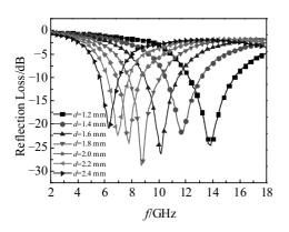
Fig.7 Reflection loss of the  $La_{0.2}Ho_{1.8}Fe_{17}$  powder with different thicknesses
