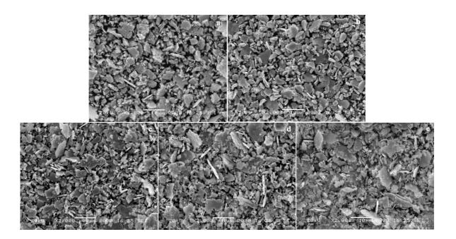
Fig.2 SEM images of the  $La_xHo_{2-x}Fe_{17}$  powders: (a) x=0.0, (b) x=0.2, (c) x=0.4, (d) x=0.6, and (e) x=0.8
