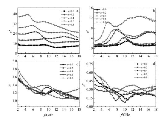
Fig.4 Electromagnetic parameters of La<sub>x</sub>Ho<sub>2-x</sub>Fe<sub>17</sub> powders with the frequency variation: (a)  $\varepsilon'$ , (b)  $\varepsilon''$ , (c)  $\mu'$ , and (d)  $\mu''$
