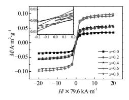
Fig.3 Magnetic hysteresis loops of the La<sub>x</sub>Ho<sub>2-x</sub>Fe<sub>17</sub> powders
