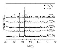
Fig.1 XRD patterns of La<sub>x</sub>Ho<sub>2-x</sub>Fe<sub>17</sub> alloys
