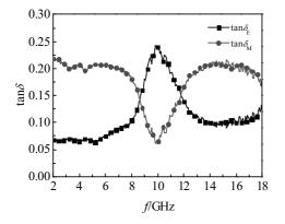
Fig.5 Relationship between loss tangent of La<sub>0.2</sub>Ho<sub>1.8</sub>Fe<sub>17</sub> powders and frequency
