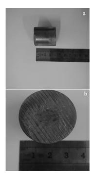
Fig.8 Size (a) and cross-section (b) of specimen after explosive consolidation
