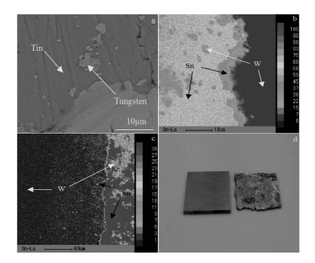
Fig.1 SEM microstructures of the diffusion-bonded joint (a); Sn mapping of interface zone for the cross-section specimens sintered at 600 °C (b) and 800 °C (c) by EPMA; unsintered and sintered (800 °C) specimens (d)
