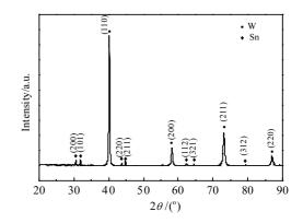
Fig.6 XRD pattern of tungsten-tin composite powder sintered at 300 °C with alkaline solution
