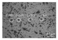
Fig.10 Variations of microhardness of the specimen
