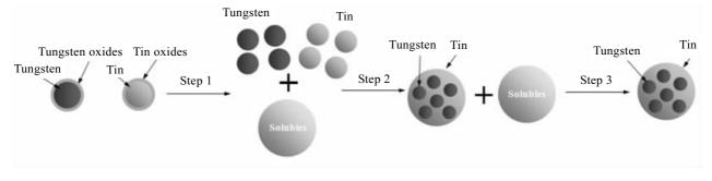
Fig.2 Schematic of the encapsulating process
