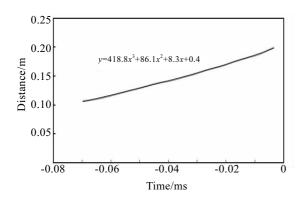
Fig.4 Distance-time curve of the detonation wave
