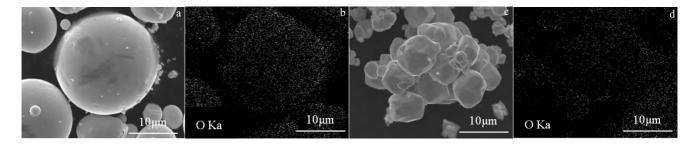
Fig.5 SEM image of tin particles (a); O mapping of tin particles (b); SEM image of tungsten particles (c); O mapping of tungsten particles (d)
