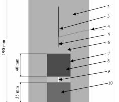
1 detonator; 2 explosive; 3 continuous velocity probe; 4 wire; 5 support structure of continuous velocity probe; 6 steel; 7 steel tube; 8 tungsten-tin alloy particles; 9 venthole; 10 steel block
