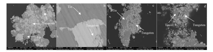
Fig.7 SEM images of specimen sintered at 300 °C with alkaline solution (a, b) and at 800 °C without alkaline solution (c, d)
