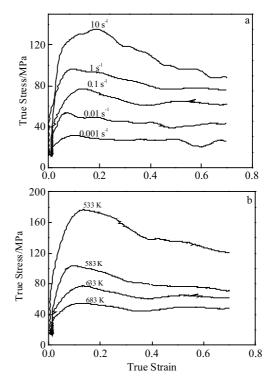
Fig.1 True stress-strain curves of AZ80 magnesium alloy at a deformation temperature of 633 K (a) and a strain rate of  $0.1 \text{ s}^{-1}$  (b)
