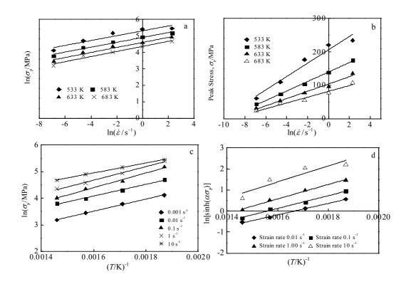
Fig.4 Curves of peak stress and strain and deformation temperature: (a)  $\ln \sigma_p - \ln \dot{\epsilon}$ , (b)  $\sigma_p - \ln \dot{\epsilon}$ , (c)  $\ln (\sigma_p) - 1/T$ , and (d)  $\ln [\sinh(\alpha \sigma_p)] - 1/T$
