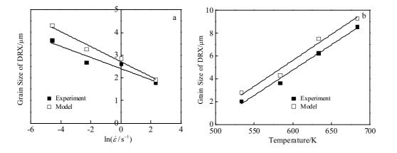
Fig.5 Comparison of the calculated and experimental results of grain size of DRX at a deformation temperature of 583 K (a) and a strain rate of  $0.01 \text{ s}^{-1}$  (b)
