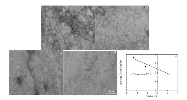
Fig.2 Microstructures of AZ80 alloy at deformation temperature of 583 K under different strain rates: (a) 0.01 s<sup>-1</sup>, (b) 0.1 s<sup>-1</sup>, (c) 1 s<sup>-1</sup>, and (d) 10 s<sup>-1</sup>; (e) average grain size vs strain rate
