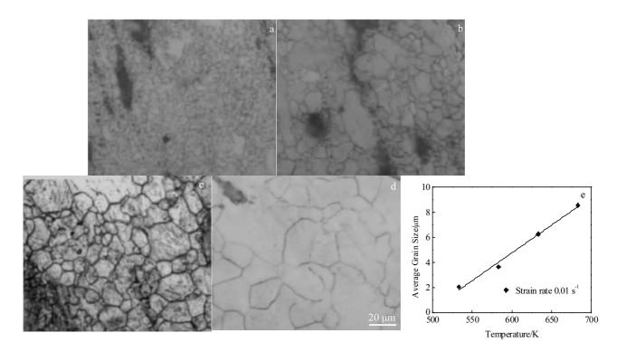
Fig.3 Microstructures of AZ80 alloy at strain rate of 0.01 s<sup>-1</sup> and different temperatures: (a) 533 K, (b) 583 K, (c) 633 K, and (d) 683 K; (e) average grain size vs deformation temperature
