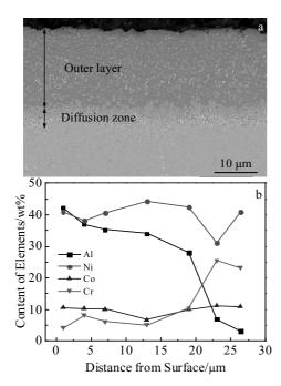
Fig.2 Cross-sectional SEM image (a) and major elemental concentration distribution (b) of the coating
