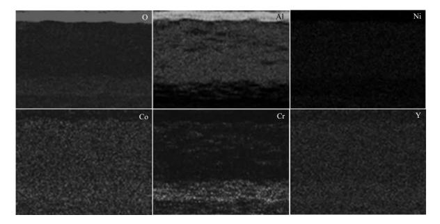
Fig. 10 EDS element mapping of O, Al, Ni, Co, Cr, Y for Cr-Co-Y-modified aluminide coating after oxidation at 1000 °C for 100 h
