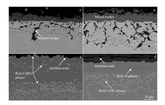
Fig.6 Cross-sectional images of the substrates (a, b) and coatings (c, d) after oxidation at 1000 °C for 20 h (a, c) and 100 h (b, d)
