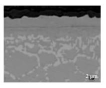
Fig. 9 SEM image of Cr-Co-Y-modified aluminide coating after oxidation at 1000 °C for 100 h
