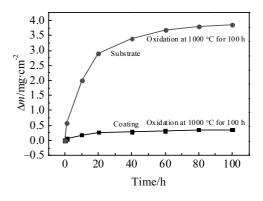
Fig.3 Isothermal kinetics of the matrix and coating specimens at 1000  $\,^{\circ}\mathrm{C}$
