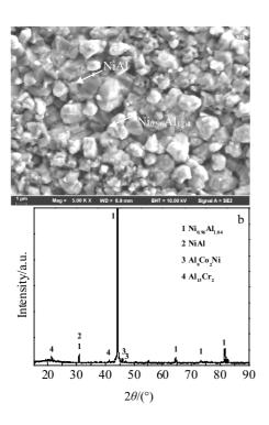
Fig.1 Surface morphology (a) and XRD pattern (b) of coating 6#
