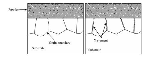
Fig.8 Mechanism of rare earth promoting the formation of aluminum coatings
