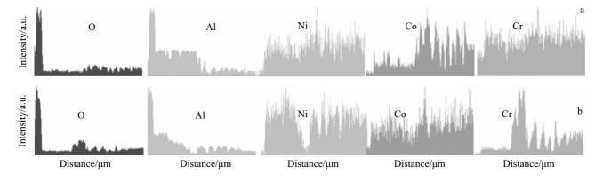
Fig.7 EDS element distributions of coatings after oxidation for 20 h (a) and 100 h (b)
