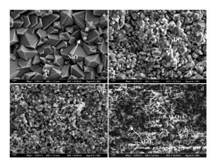
Fig.4 SEM morphologies of the substrate surfaces (a, b) and coatings (c, d) after oxidation at 1000 °C for 20 h (a, c) and 100 h (b, d)
