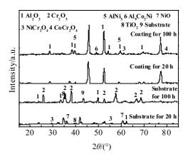
Fig.5 XRD patterns of the substrate and the coating surface after oxidation at 1000 °C for 20 and 100 h
