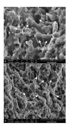
Fig.7 Fracture surface of Al/B<sub>4</sub>C composites prepared by different processes: (a) vacuum sintering and (b) semisolid HIP
