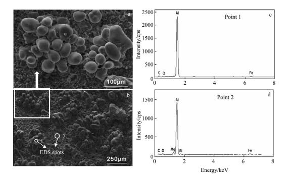
Fig.5 SEM images (a, b) and EDS spectra (c, d) of the free surface of Al/B4C composites
