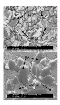
Fig.2 Microstructures of Al/B<sub>4</sub>C composites prepared by conventional vacuum sintering (a) and semisolid HIP (b)
