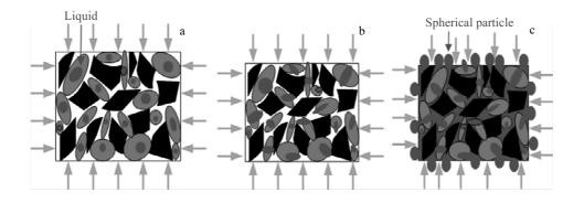
Fig.6 Proposed densification mechanism of semisolid HIP: (a) liquid phase appears, (b) liquid phase overflows, and (c) spherical particles appear
