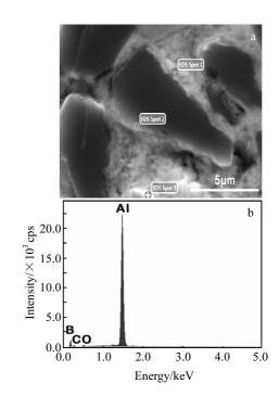
Fig.3 SEM image (a) and EDS spectrum (b) of Al/B<sub>4</sub>C composites prepared by semisolid HIP
