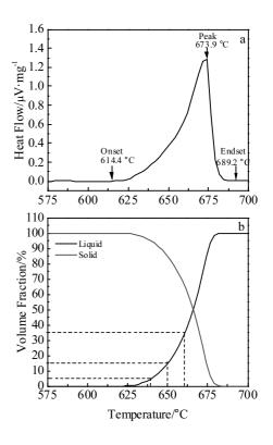
Fig.1 DSC curve of 6061 Al alloy powders at a heating rate of 10 °C/min (a) and volume fraction of solid and liquid versus temperature derived from the DSC curves (b)
