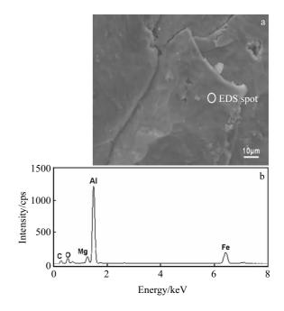
Fig.4 SEM morphology (a) and EDS analysis (b) of the surface of Al/B<sub>4</sub>C composites prepared by semisolid HIP
