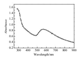
Fig.1 Typical UV-visible spectrum of the nano gold colloids
