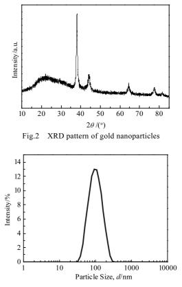
Fig.3 Particle size distribution of gold nanoparticles by intensity
