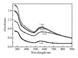
Fig.8 UV-vis spectra of gold colloids synthesized at different amount of leaf extract
