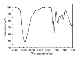
Fig.7 FT-IR spectrum of the prepared gold nanoparticles
