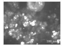
Fig.4 Typical SEM image of gold nanoparticles
