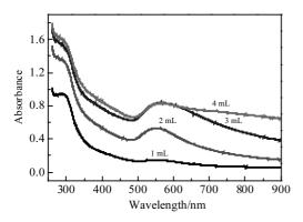
Fig.9 UV-vis spectra of gold colloids synthesized with different amounts of chloroauric acid amount solution
