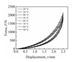
Fig.6 Hysteretic curves of common-MR at different temperatures
