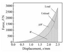
Fig.3 Hysteresis loop of the SMA-MR damping
