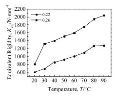
Fig.7 Equivalent rigidity curves of SMA-MR at different temperatures
