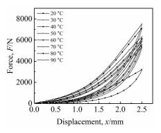
Fig.5 Hysteretic curves of SMA-MR at different temperatures
