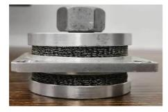
Fig.2 Picture of the SMA-MR damper
