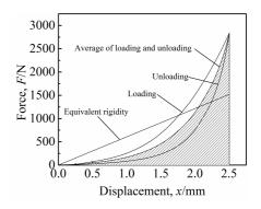
Fig.4 Solution principle of equivalent rigidity curve
