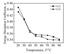
Fig.8 Energy dissipation coefficient-temperature curves of SMA-MR dampers
