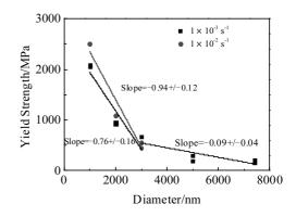
Fig.5 Relationship between yield strength of <110>-oriented singlecrystalline iridium micropillars and micropillar diameters
