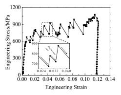
Fig.2 Engineering stress-strain curve of iridium micropillars with 3000 nm in diameter (inset displaying three zoomed-in displacement jumps)
