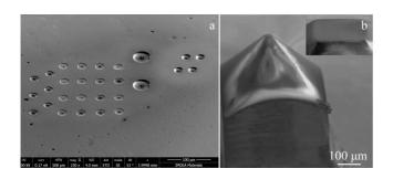
Fig.1 <110>-oriented single-crystalline iridium micropillars with different sizes (a) and SEM image of diamond indenter (b)
