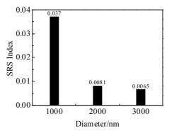
Fig.6 Relationship between SRS index (*m*) and diameters for <110>- oriented single-crystalline iridium micropillars
