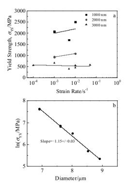
Fig.4 Yield strength of <110>-oriented single-crystalline iridium micropillars as a function of strain rate (a) and relationship between yield strength and diameters at the strain rate of  $1 \times 10^{-3}$  s<sup>-1</sup> (b)
