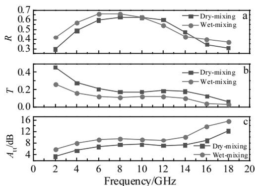
Fig.5 Absorbing characteristics of MWCNTs/TiO<sub>2</sub>: (a)  $R$ -reflectance curves, (b)  $T$ -transmittance curves, and (c)  $A_u$ -attenuation curves
