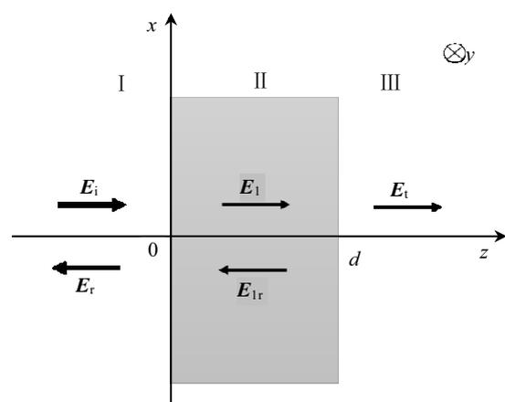
Fig.1 Physical model of electromagnetic wave propagation in absorber with MWCNTs/TiO<sub>2</sub> composite powder particles distribution: I-Air, II-Absorber, III-Air;  $E_i$  is the incident wave,  $E_r$  is the reflection wave,  $E_{1i}$  is the transmission wave entering the absorber,  $E_{1r}$  is the reflection wave coming from the absorber, and  $E_t$  is the transmission wave
