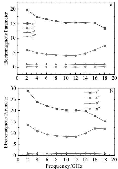
Fig.4 Electromagnetic parameters of dry mixed MWCNTs/TiO<sub>2</sub> (a) and wet mixed MWCNTs/TiO<sub>2</sub> (b)
