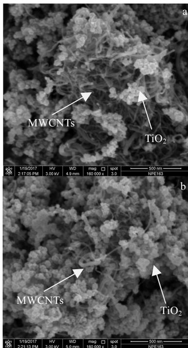
Fig.3 SEM images of dry-mixed (a) and wet-mixed (b) MWCNTs/TiO<sub>2</sub> samples
