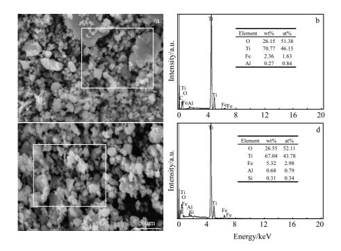
Fig.5 Morphologies (a, c) and EDS results (b, d) of wear debris of pure Ti (a, b) and Ti alloys with 0.5 wt% RHAs SiO<sub>2</sub> (c, d)
