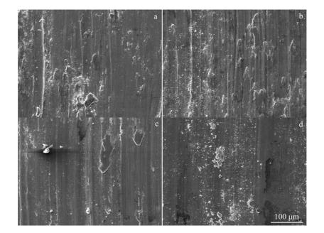
Fig.4 Worn surface of Ti alloys with different RHAs SiO<sub>2</sub> addition: (a) 0 wt%, (b) 0.25 wt%, (c) 0.5 wt%, and (d) 1.0 wt%
