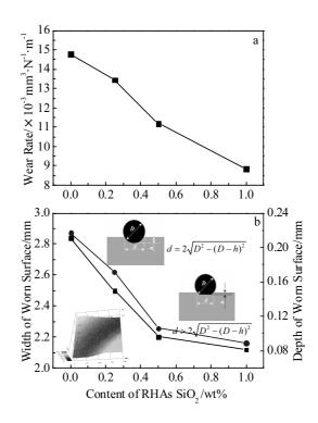
Fig.3 Volume wear rate (a) and geometric size (b) of worn groove of Ti alloys with different RHAs SiO<sub>2</sub> addition (3D LSCM profile of the worn surface is inserted in Fig.3b)
