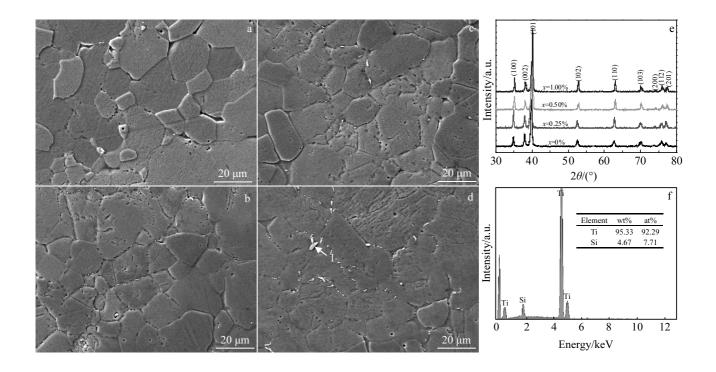
Fig.1 Microstructures of Ti alloys with different content of RHAs SiO<sub>2</sub> addition: (a) 0 wt%, (b) 0.25 wt%, (c) 0.5 wt% and (d) 1.0 wt%; XRD patterns (e) and EDS result (f) of the white particle marked by arrow "1" in Fig.1d
