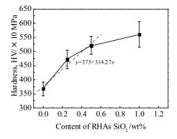
Fig.2 Hardness of Ti alloys with different RHAs SiO<sub>2</sub> contents
