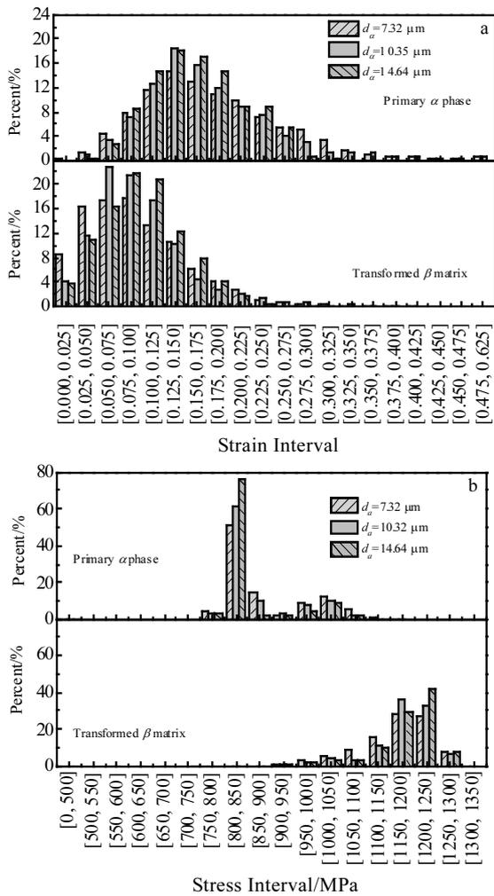
Fig.8 Effect of  $\alpha_p$  grain size on train (a) and stress (b) distributions
