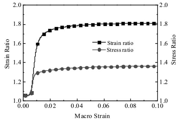
Fig.5 Variation curves of strain and stress ratios with macro strain
