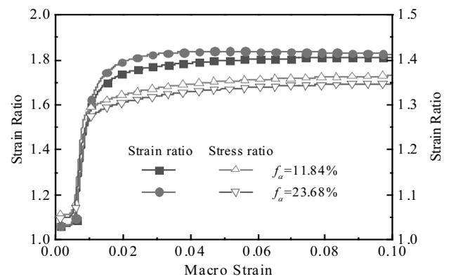
Fig.7 Effect of volume fraction of  $\alpha_p$  on strain and stress ratios
