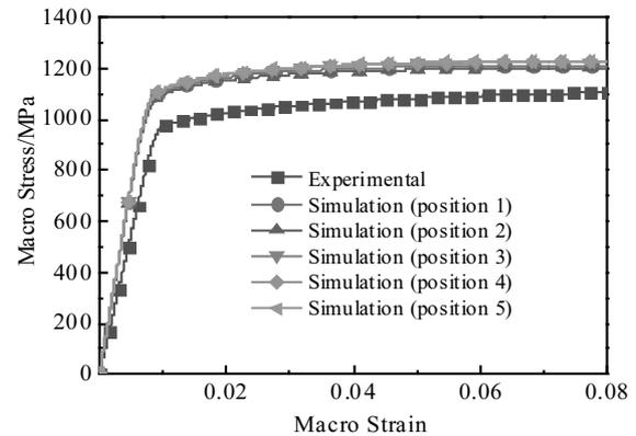
Fig.3 Effect of microstructures in different regions on simulation results of stress-strain curves for Ti-6Al-4V alloy
