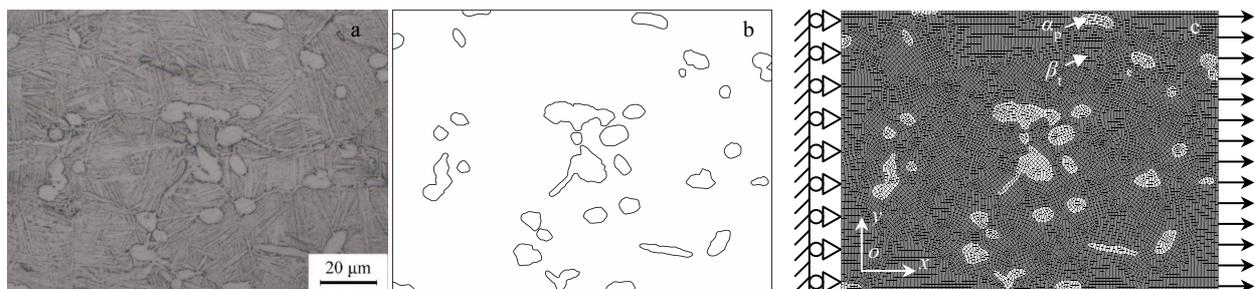
Fig.1 Metallographic microstructures of the heat treated titanium alloy (a), vectorized boundary lines of the model (b), and mesh and boundary condition of the model (c)
