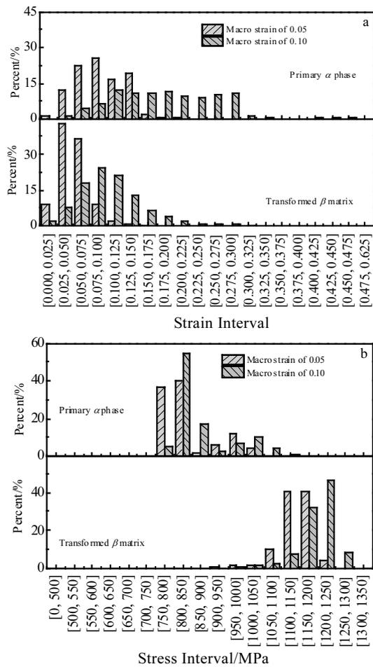
Fig.4 Quantitative statistics for strain distribution (a) and stress distribution (b) in constituent phases
