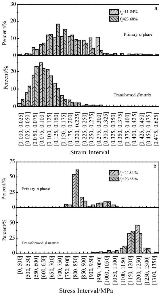
Fig.6 Effect of volume fraction of  $\alpha_p$  on strain distribution (a) and stress distribution (b) of constituent phases
