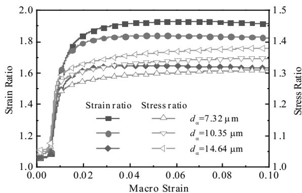
Fig.9 Effect of  $\alpha_p$  grain size on strain and stress ratios
