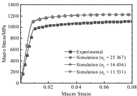
Fig.2 Effect of mesh quantity on simulation results of stress-strain curves for Ti-6Al-4V alloy
